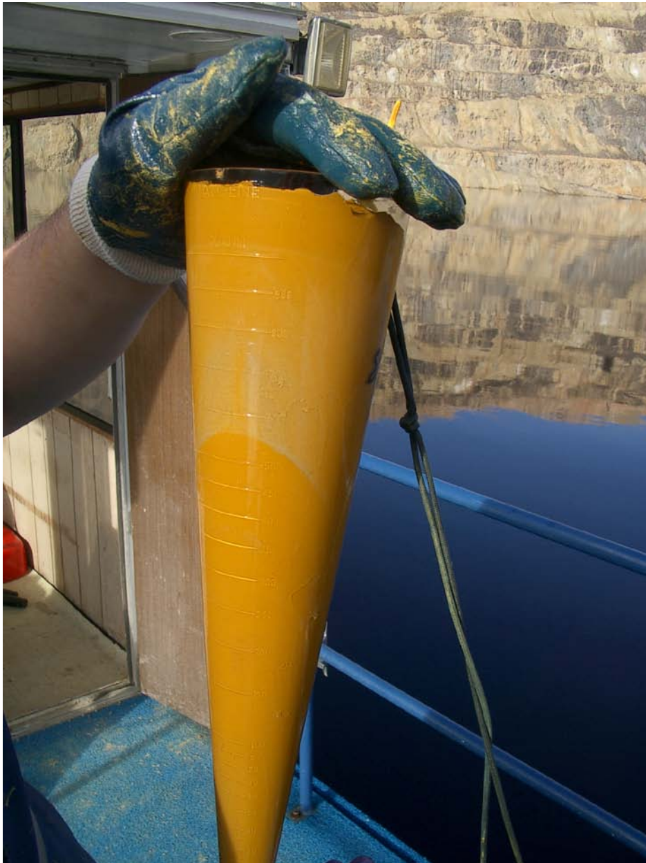
Figure 2-50. Accumulation of secondary iron precipitates in a sediment trap deployed in the Berkeley Pit for 150 days.
