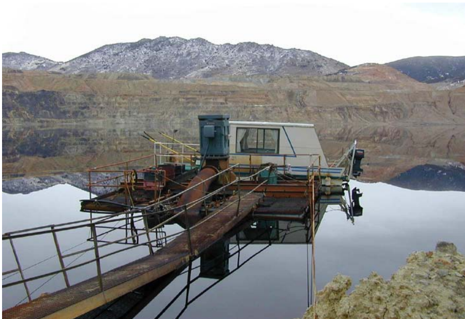
Figure 2-46. MR pontoon boat is used for Berkeley Pit sampling. Boat is docked next to pump station used for pumping pit water to precipitation plant for copper recovery. (Photo courtesy of Daryl Reed, DEQ)
