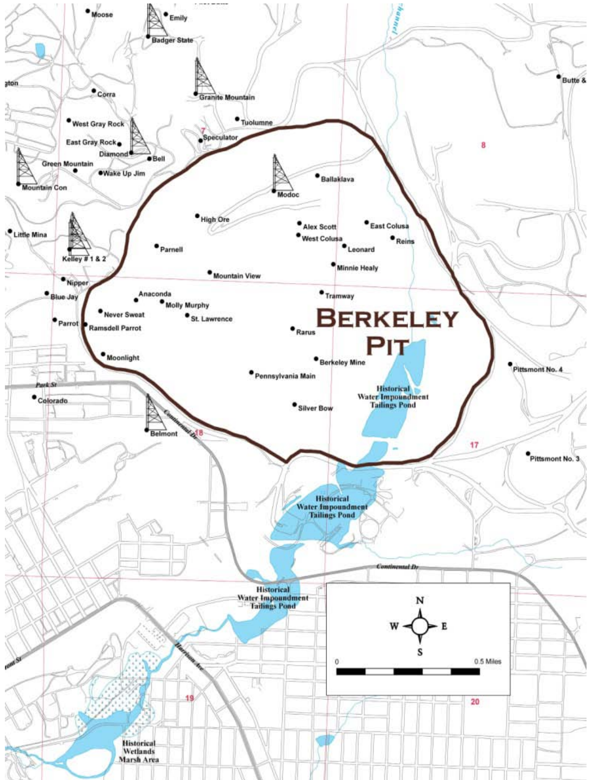
Figure 1-1. Map showing location of selected underground mines engulfed by development and expansion of the Berkeley Pit.
