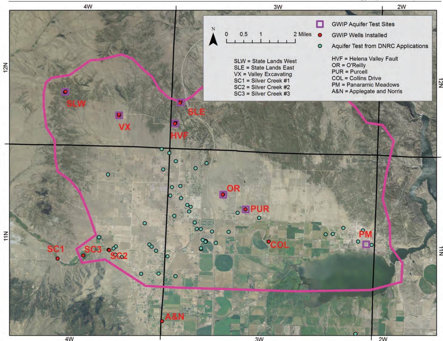
Figure 13. Wells were installed and aquifer tests were conducted at various locations within the North Hills Study Area to acquire water-level information and to evaluate aquifer properties. Aquifer test data from DNRC applications (P. Faber, written commun., 2010) also provided significant additional information on aquifer properties.
