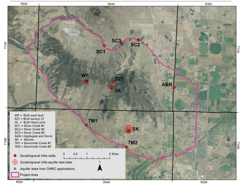
Figure 7. Wells were installed at 10 locations within the Scratchgravel Hills study area to acquire water-level information and to evaluate aquifer properties. Six aquifer tests were conducted. Aquifer test data from numerous DNRC water-rights applications also provided information on aquifer properties.
