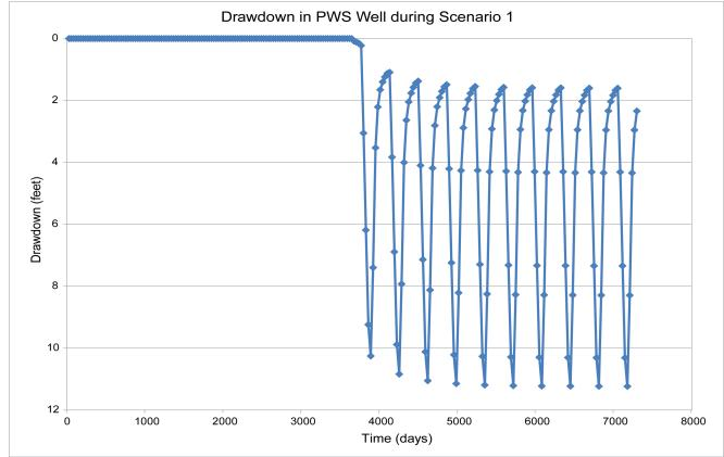
Figure 24. Scenario 1 illustrates modeled drawdown from a public water supply well located in the SE½SE½NE½ sec. 11, T. 10 N., R. 4 W., designed to provide water to 33 homes on 10-acre lots. This well is completed in the alluvium. The well's maximum radius of influence extends about 0.5 mile (A), its maximum drawdown is approximately 11 ft, and water levels stabilize during the 10-yr model run (B).
