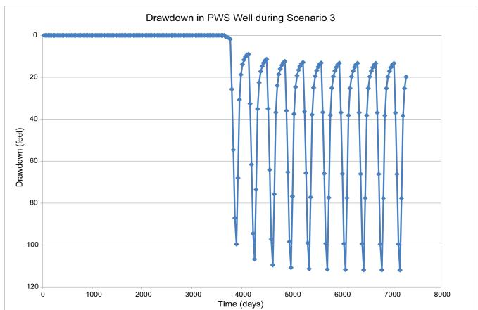
Figure 26. Scenario 3 illustrates modeled drawdown from a public water supply well located in the SE½SE½NE½ sec. 11, T. 10 N., R. 4 W., designed to provide water to 267 homes on 1.2-acre lots. This well is completed in the alluvium. The well's maximum radius of influence extends about 1.3 miles (A), maximum drawdown is approximately 112 ft, and water levels stabilize during the model run (B).
