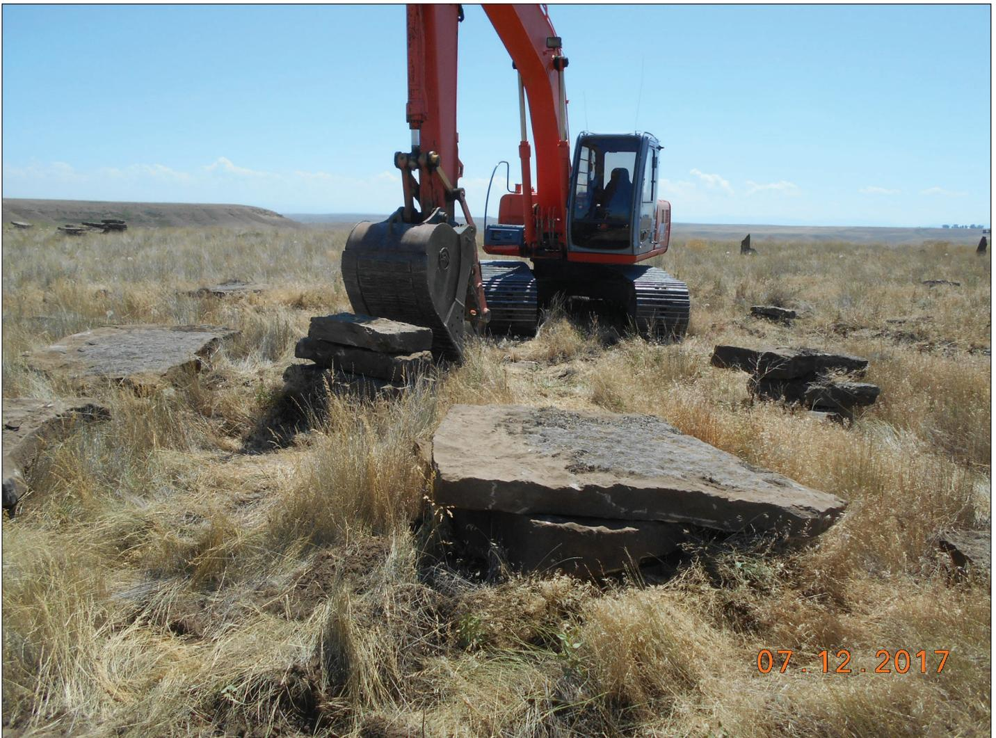
Figure 3. An excavator is used to remove slabs of sandstone from shallow depths in a field north of Vaughn. The stone is hauled to another location to be sorted and shaped. The ground disturbance is then graded and seeded to establish vegetation.
