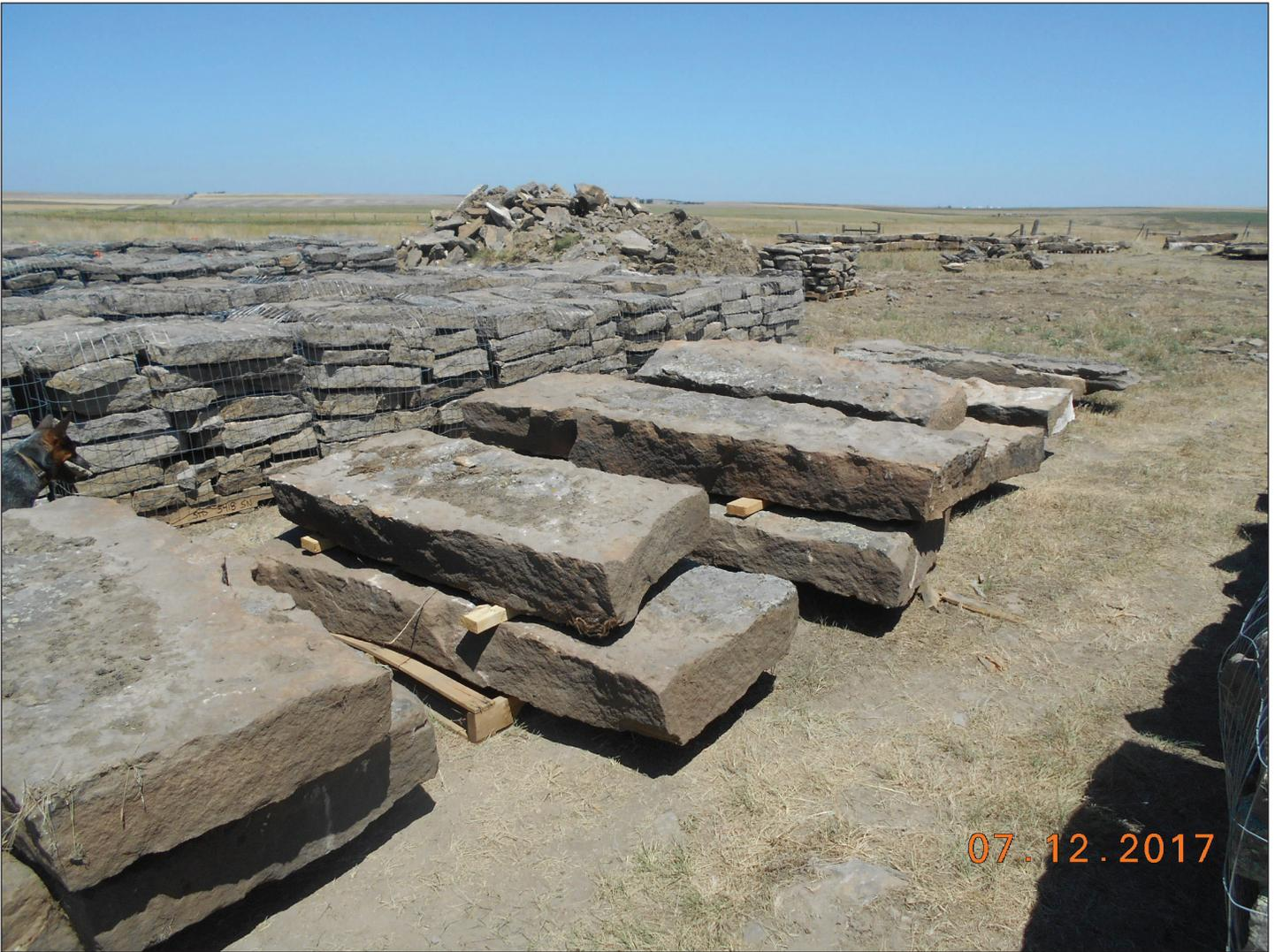
Figure 4. Depending on market demands, the larger rock slabs may be sold directly or they may be sized and shaped with a pneumatic rock chopper before being stacked on pallets for shipping.
