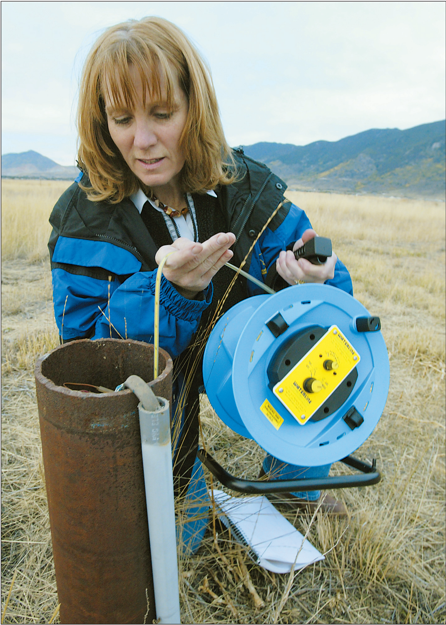
HYDROGEOLOGIST KATE MILLER MEASURES the water depth of a well on her property south of Butte using a water-level indicator. The bureau has 15 hydrogeologists on staff, working on water quality and supply projects across Montana.
