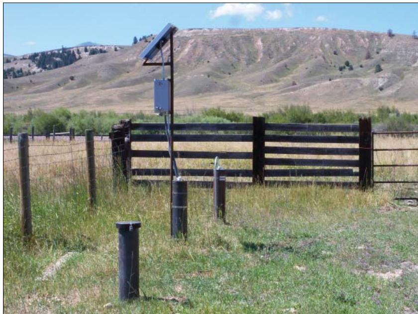
In an effort to improve efficiency and provide timelier water-level data from critical locations, the Ground Water Monitoring Program has installed three telemetry units to gather and send data directly to the Ground Water Information Center database. A photograph of the Deer Lodge Valley telemetry site is at top right.
