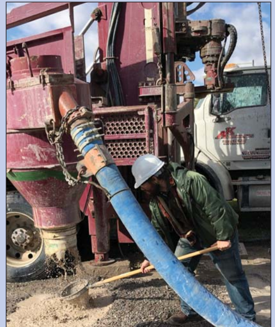
Collecting drill cuttings to identify aquifers in the Flathead Valley.
