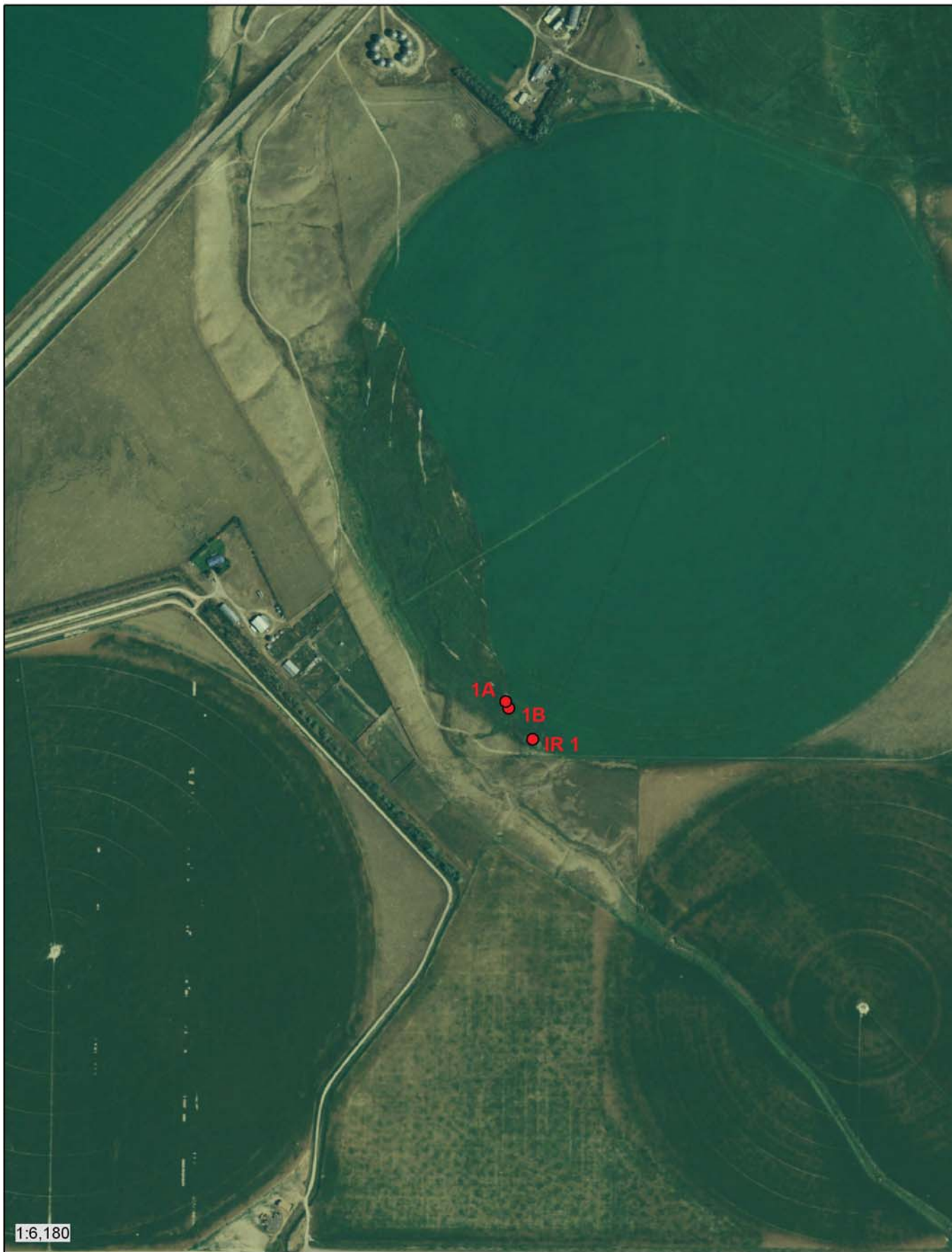
Figure 9. Aerial photograph showing the locations of wells 1A and 1B drilled to monitor the effects of pumping from a nearby irrigation well (IR1). Irrigation monitoring well site shown in figure 5.
