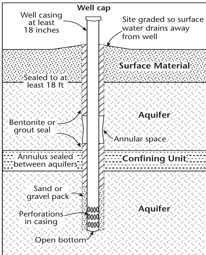
Figure G-8. Properly constructed wells are completed in single aquifers. In order to protect ground-water quality and maintain artesian pressures, wells should not serve as conduits from the surface to ground water or connect separate aquifers.
