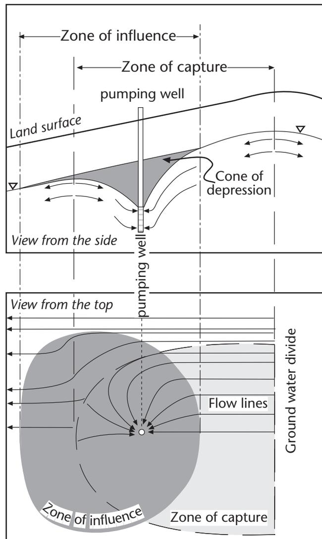
Figure G-9. Withdrawal of ground water will temporarily depress the water level (potentiometric surface) in the region surrounding the well, creating a "cone of depression." The dimensions of the cone of depression, zone of influence, and zone of contribution depend on hydraulic characteristics of the aquifer, potentiometric surface, and discharge rate of the well.
