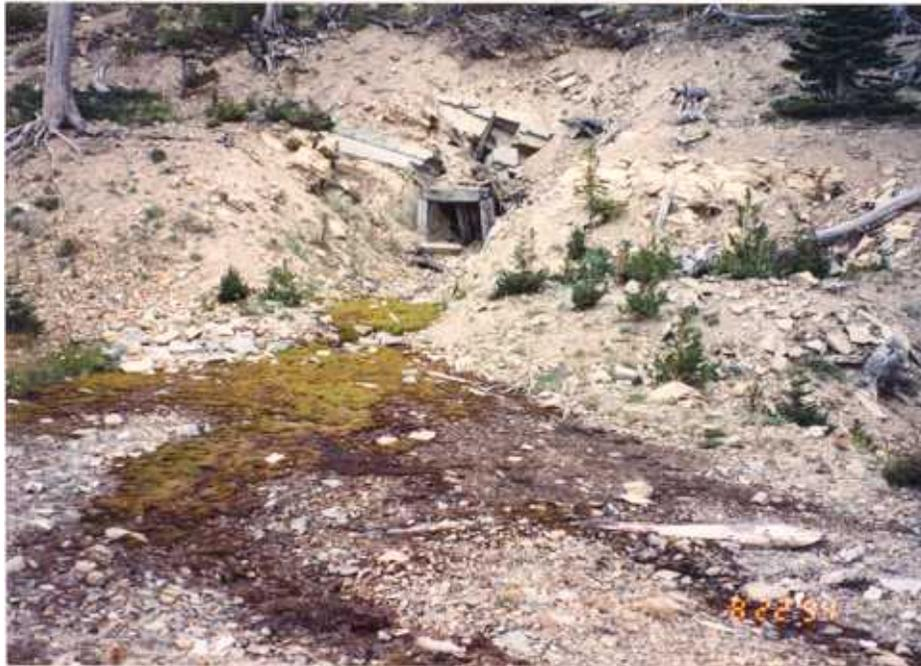
Figure 29a. Upper Copper Camp adit, trended N15°E, with <five-gpm discharge that infiltrated into dump.
