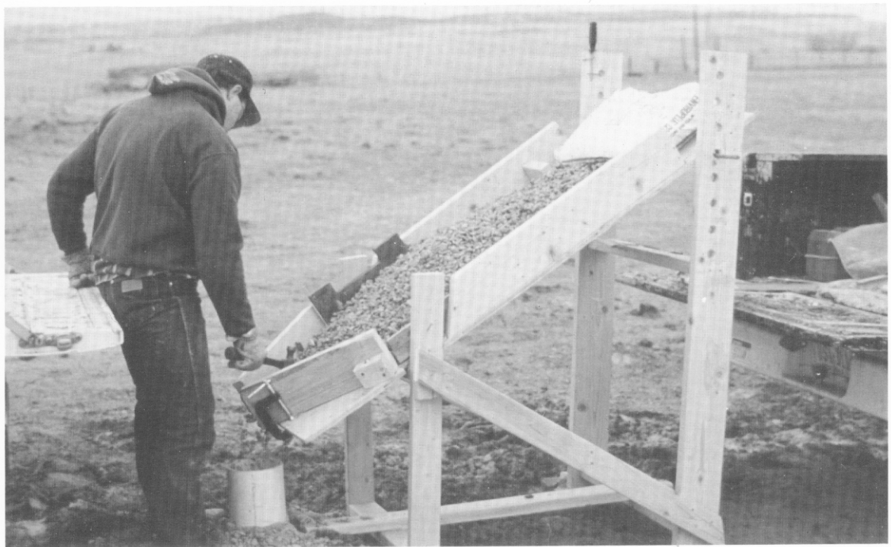
Figure 6—Two types of pour-rate control apparatus were used. The PVC funnel (top) performed acceptably with \frac{3}{8} -inch chips, but occasionally bridged. The wooden chip tray (bottom) provided maximum flexibility with different chip sizes.
