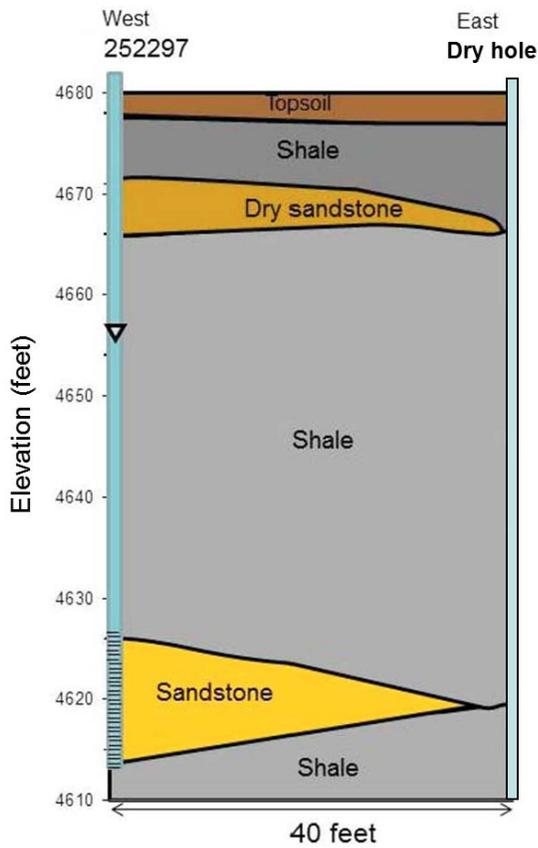
Figure 38. Well completion diagram for a well (252297) drilled into the Hell Creek aquifer.
