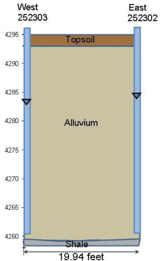
Figure 21. Well completion diagram for observation well 252303 and pumping well 252302. Water levels used for the diagram were measured on 8-25-09.
