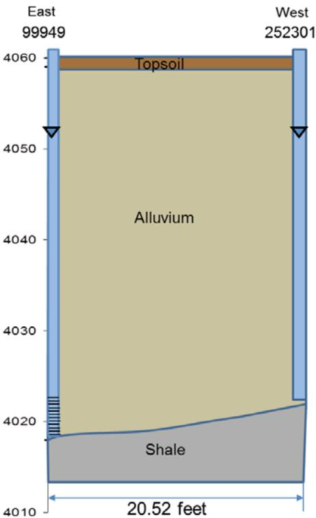
Figure 15. Well completion diagram for observation well 99949 and pumping well 252301. Water levels used for the diagram were measured on 8-25-09.
