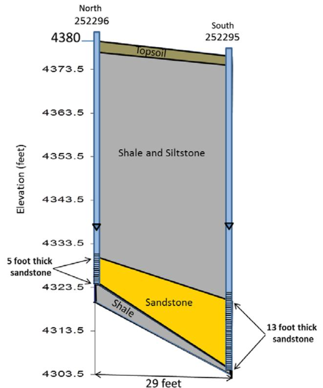
Figure 35. Well completion diagram for wells (252296, 252295) drilled into the Tullock aquifer.
