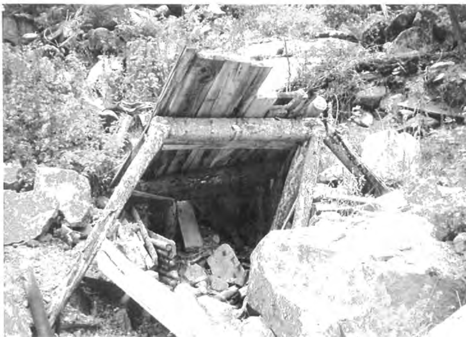
Figure 6.4 Adit "A02" trends N60°E and has a small discharge barely discernable in the lower center of photo.
