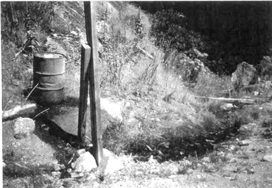
Figure 7.15 At the Garnet Gold mine, waste-oil(?) leaking from a 55-gallon drum has stained the soil near the adit.
