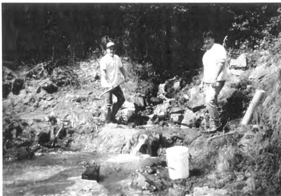
Figure 6.13 At sample location FLKS20H, technicians Frank Carr and Todd Werner measured the flow rate of the stream using a pipe dam, bucket, and stopwatch.
