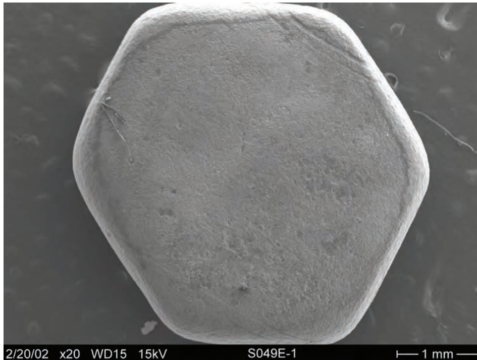
Figure 13. Observation —A few sapphires retain their original prismatic crystallographic form, as does this tablet with a prominent basal surface. The grooves in the upper right corner of the tablet were formed by resorption, probably along the rhombohedral twinning. Interpretation —Minor etching occurred during transport in magma.
