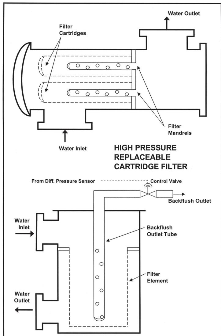
Figure 10. Cartridge type filters.
