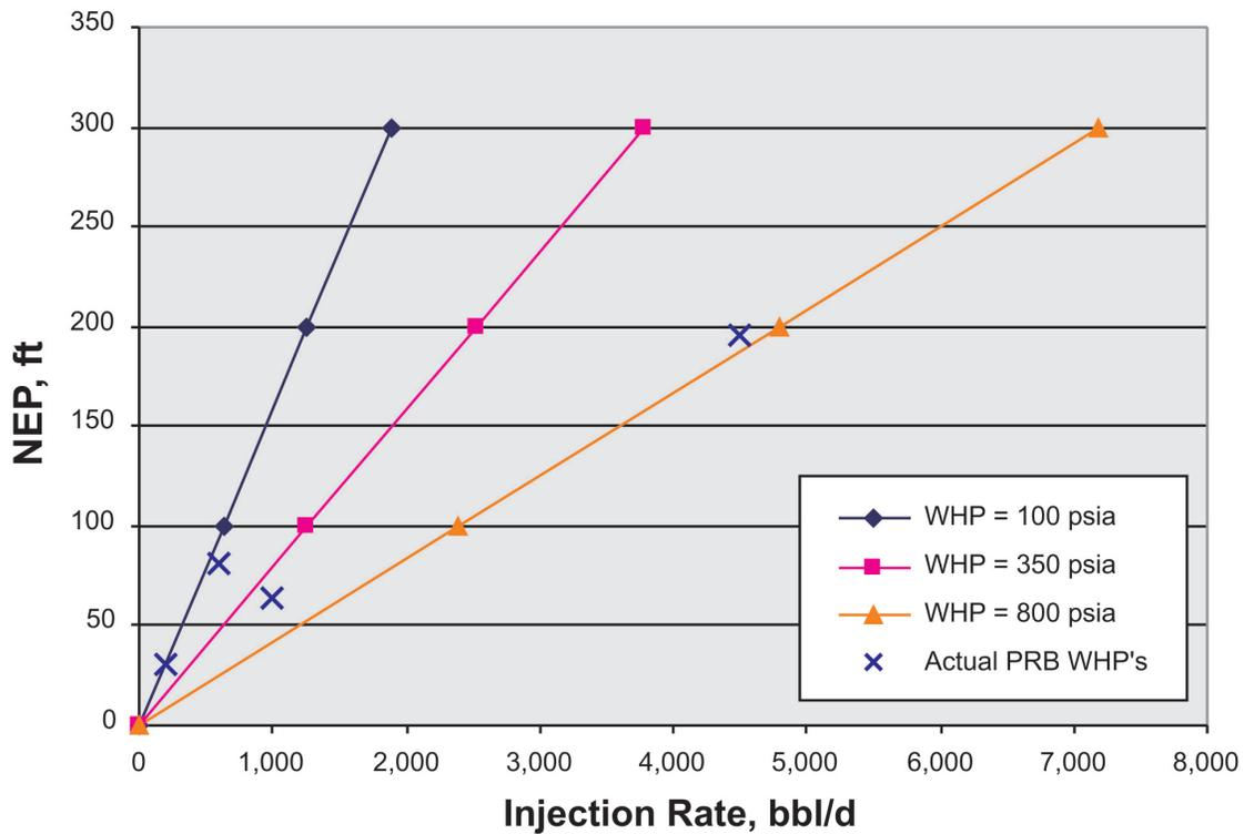
Figure 8. Expected water injection rates vs. zone thickness and wellhead pressure.
