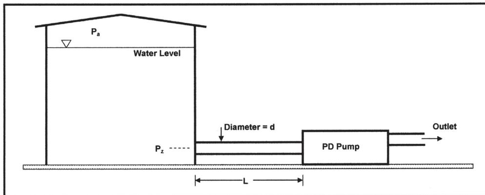
Figure 12. Typical water pumping system.
