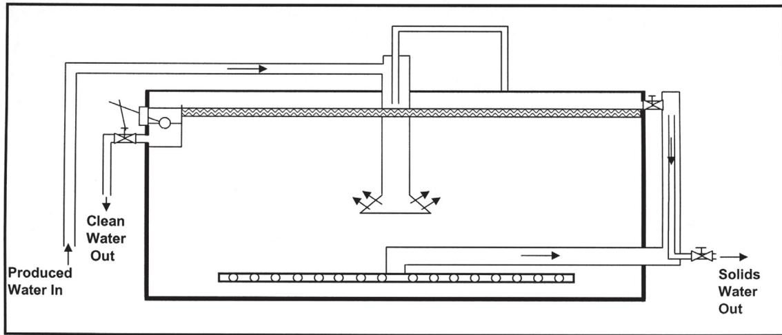
Figure 9. Skimmer and sedimentation tank.
