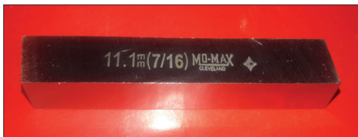
Figure 2. A Co cutting tip used in millwork to shape metals. Photo by Metrónomo (CC-BY-SA-4.0)
