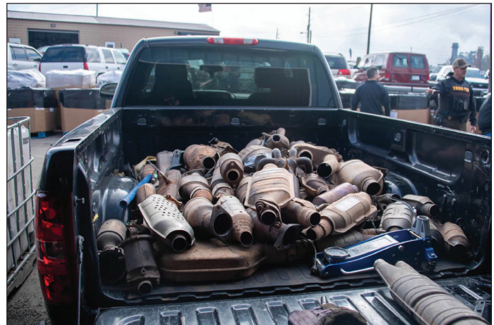
Figure 2. A truckload of stolen Pt-containing catalytic converters seized by law enforcement. These components have a ceramic honeycomb interior sprinkled with PGEs that engine exhaust passes through. The gases are made less toxic by way of chemical reactions catalyzed by the PGEs. Due to the high value of PGEs, such thefts are common. Photo by Department of Homeland Security (CC-PD-Mark).
