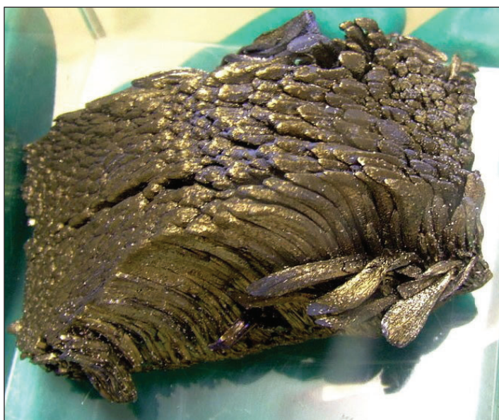
Figure 1. 300 grams of refined Eu metal held in hand. Photo by Alchemist-hp (CC-BY-SA-3.0-DE).
