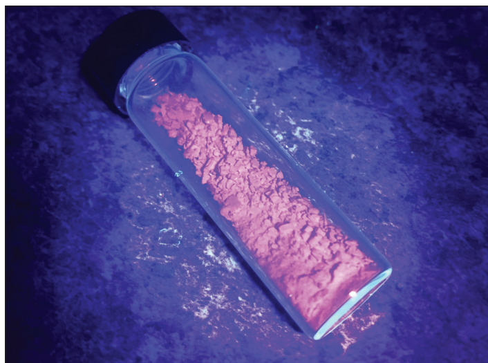
Figure 2. Eu hydroxide under ultraviolet light, glowing with a red-dish color that distinguishes many Eu compounds. Photo by Leo S. (CC-BY-SA-4.0).
