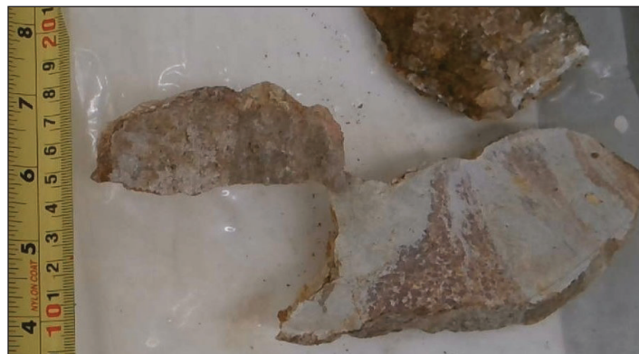
Figure 3. A sample of REE-mineralized carbonatite with ~0.01 wt.% Eu from Ravalli County, Montana. Photo by Adrian Van Rythoven (MBMG).
