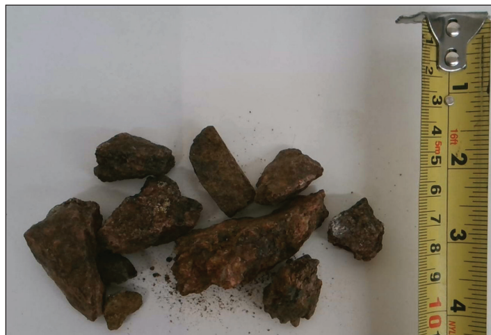
Figure 3. A sample of weathered REE-mineralized carbonatite with 0.073 wt.% Sm from Beaverhead County, Montana. Photo by Adrian Van Rythoven (MBMG).
