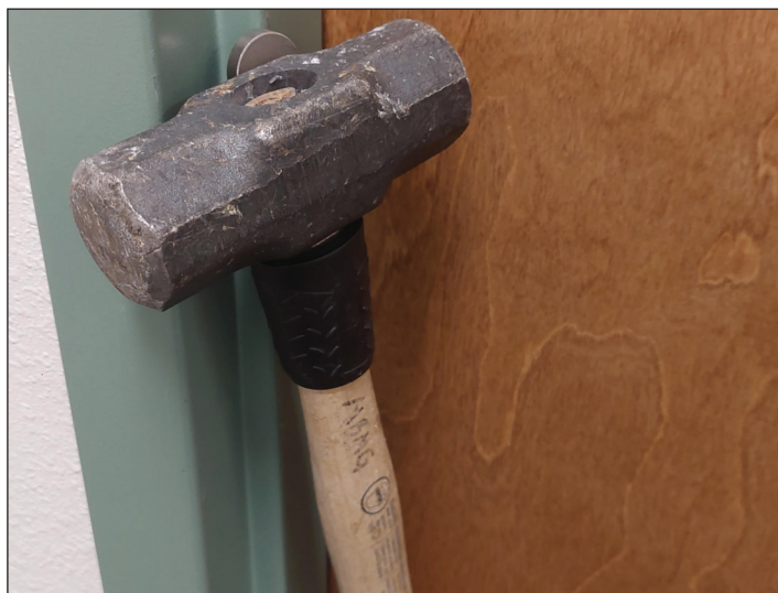
Figure 2. A cylindrical (1" x 0.25") Sm-Co magnet demonstrating its strength holding a small (~6 lbs) sledgehammer to a metal doorframe. A conventional (non-REE) ceramic magnet of the same size would not be able to hold this weight. Photo by Adrian Van Rythoven (MBMG).
