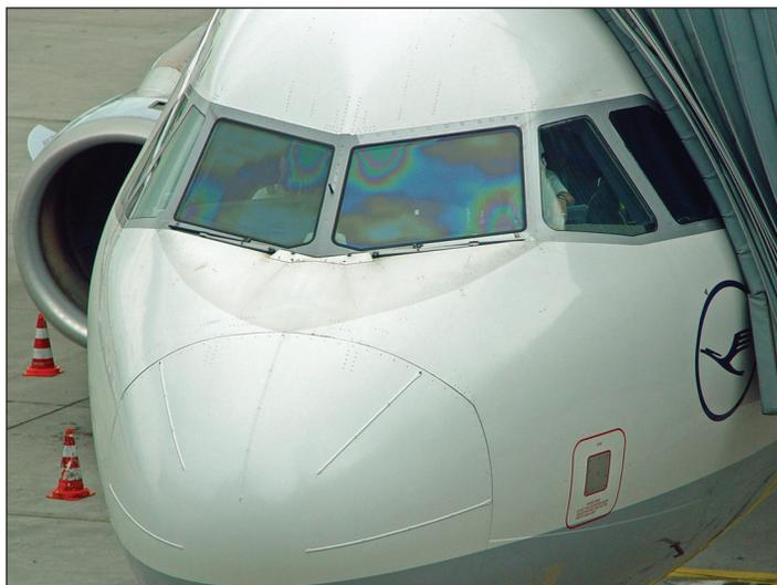
Figure 3. Optical fringes seen on the cockpit window of a commercial jetliner. The fringes are caused by an In-Sn-oxide coating that is electrically conductive to allow for controlled uniform defogging and defrosting. Photo by Etan J. Tal (CC-BY-SA-3.0).
