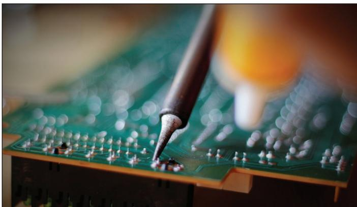
Figure 2. Electronic connections on a circuit board being soldered with Sn-based solder (CC0 1.0 Universal).
