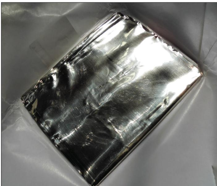
Figure 1. Thin foil of Sn metal weighing 100 grams. Photo by Leiem (CC BY-SA 4.0).
