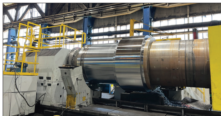
Figure 2. A component made of Cr-alloy for a Royal Navy (U.K.) nuclear submarine being machined. Photo courtesy of Michael Devlin, Evolution Metals and Mining Technologies, LLC.
