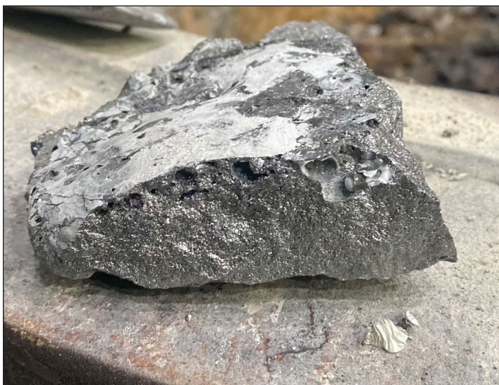
Figure 1. A piece of refined low-carbon ferrochromium alloy. Photo courtesy of Michael Devlin, Evolution Metals and Mining Technologies, LLC.
