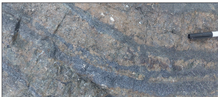
Figure 3. Bands of black chromite ore in green pyroxenite from the closed Mountain View Cr Mine, Stillwater County, Montana. Marker for scale. Photo by Adrian Van Rythoven.
