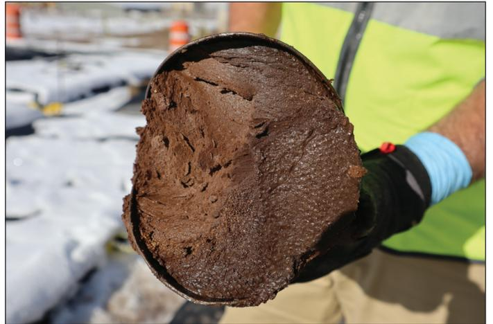
Figure 25. Geotube imprint left on HPC core bottom (Bird, in process, with permission.)
