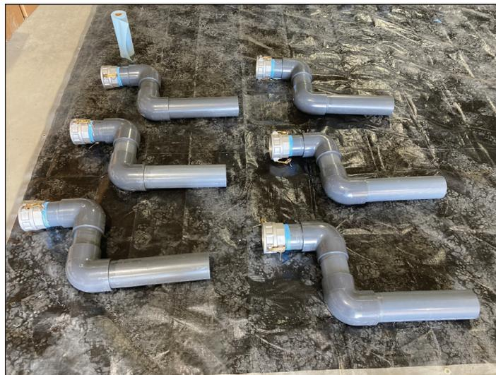
Figure 13. Assembled filling lances.
