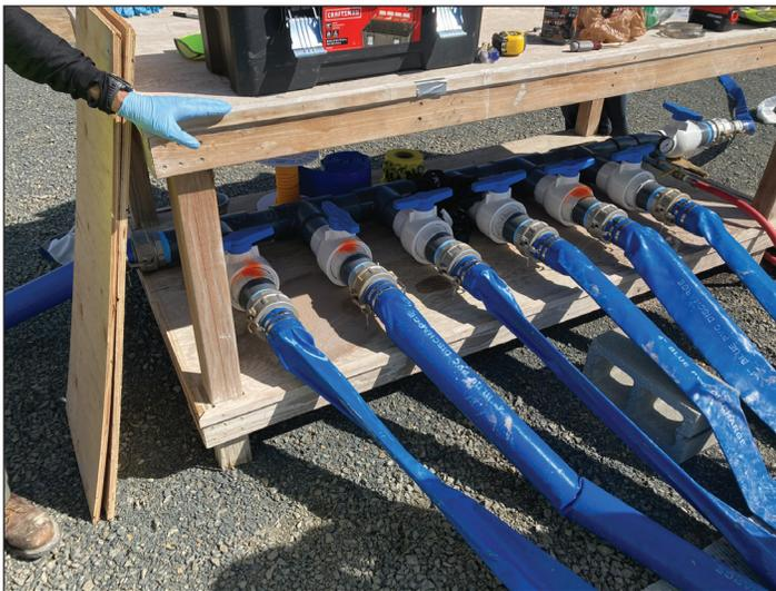
Figure 12. Assembled manifold.
