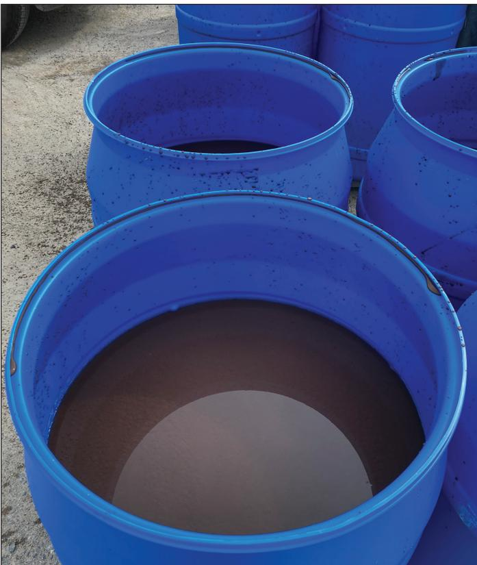
Figure 15. 55-gallon barrels of decanted REE hydraulic preconcentrate.
