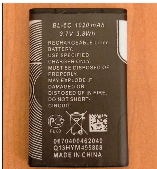
Figure 3. A 3.7 V Li-ion battery. Fluorine from fluorspar is used to create the Li-bearing electrolyte in many types of Li-ion batteries. Photo by Emilio J. Rodriguez Posada (CC-BY-SA-4.0).
