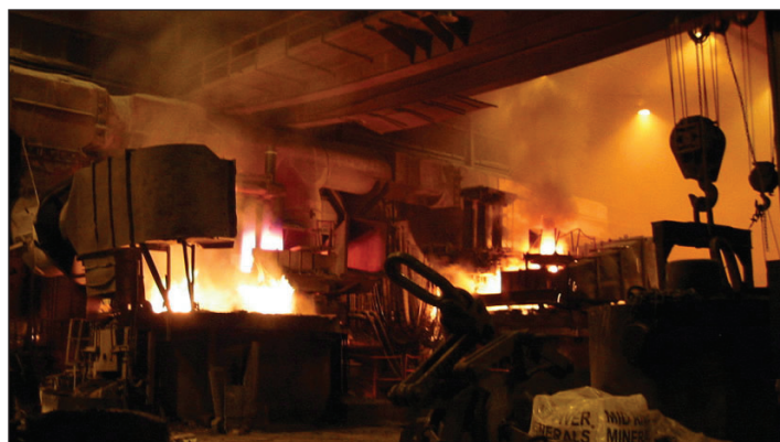
Figure 2. A photo of the Finkl Steel Mill operations near Chicago, Illinois. Low-grade fluorspar (metallurgical fluorspar) is added as a flux to help iron ore melt and to remove impurities. The white bags in the foreground likely hold fluorspar. Photo by Payton Chung (CC-BY-2.0).
