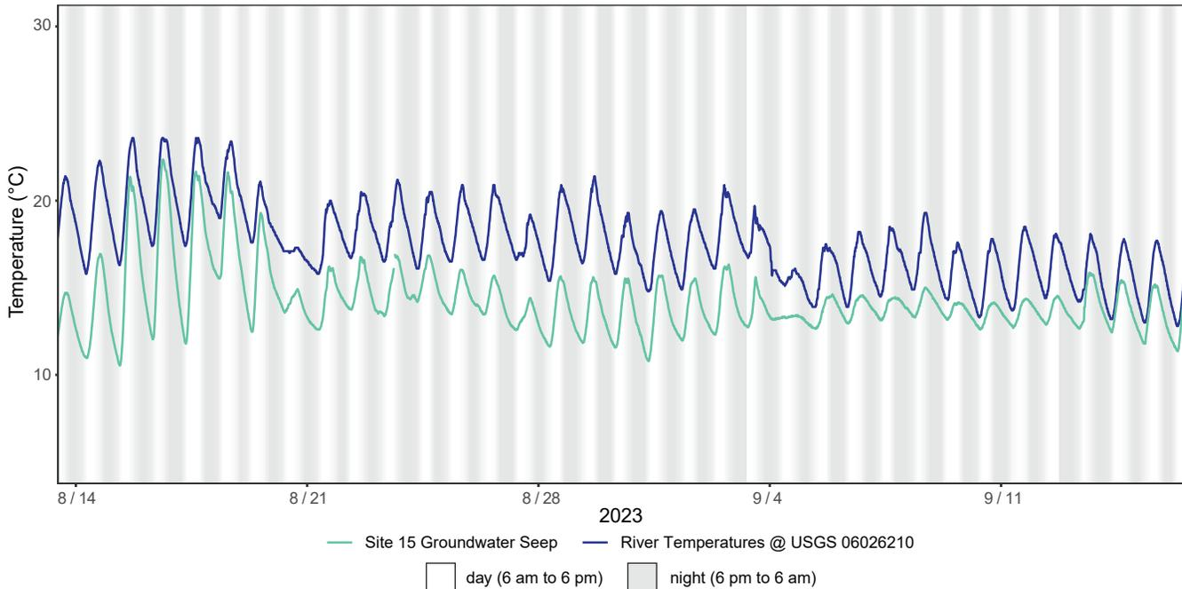
Figure A15.4. August–September 2023 logged temperatures at Site 15 groundwater seep (334300) compared to the river temperatures at the USGS gaging station Big Hole River near Glen, MT (06026210). The diel fluctuations of the groundwater seep were inconsistent, but the overall temperature was generally cooler than the river.
