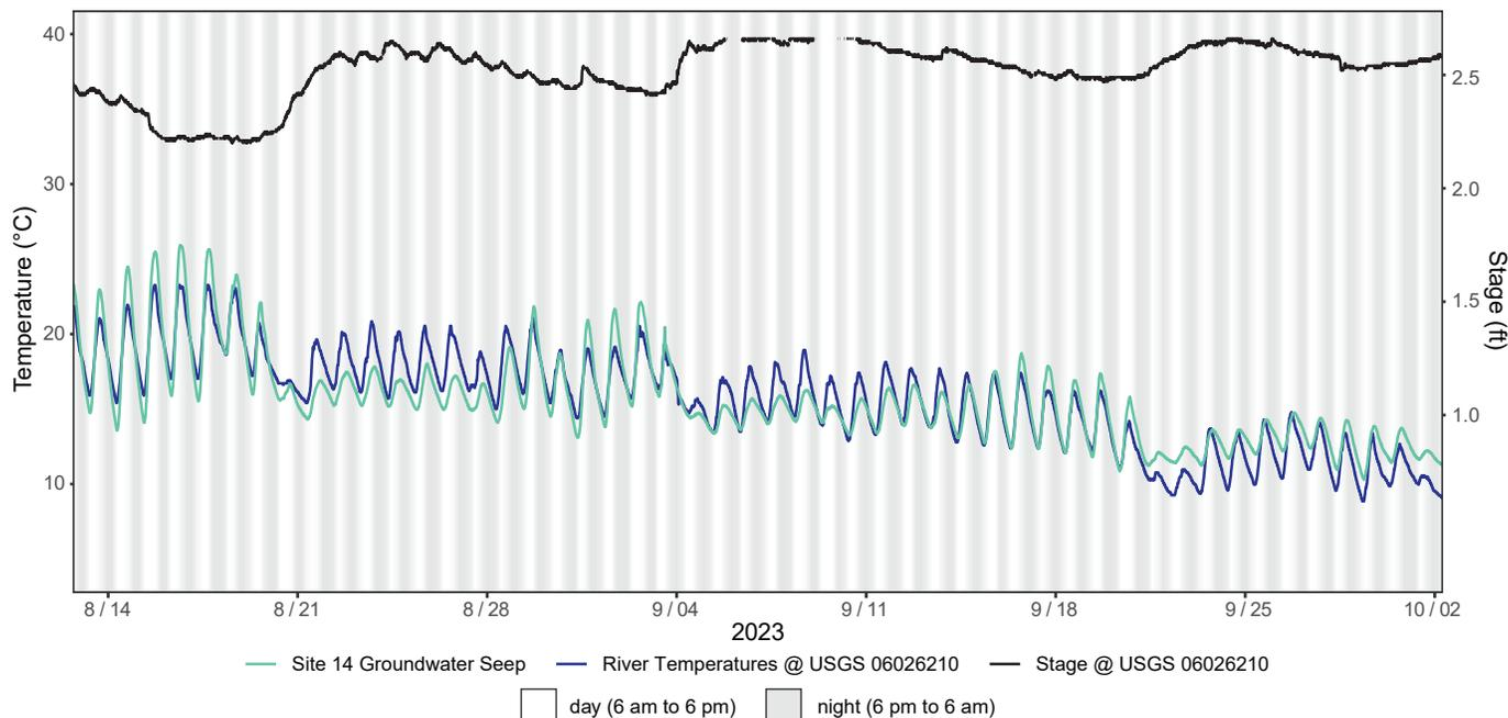
Figure A14.4. August–October 2023 logged temperatures at Site 14 groundwater seep (334299) compared to the river temperatures at the USGS gaging station Big Hole River near Glen, MT (06026210). The small amount of groundwater flow coming from the site was cooler within the saturated riverbank before entering the river during late August. Groundwater temperatures were slightly warmer than the river during late September.
