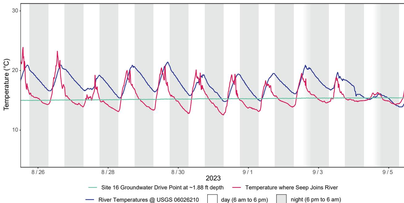
Figure A16.4. Late August to September 2023 logged temperatures at Site 16 groundwater seep (327572) compared to the river temperatures at the USGS gaging station Big Hole River near Glen, MT (06026210). Temperature was also monitored where the ponded groundwater reached the river (~200 ft away; 334301) which was commonly warmer than the river during midday after flowing along the surface of the gravel bar (see fig. 16.2).
