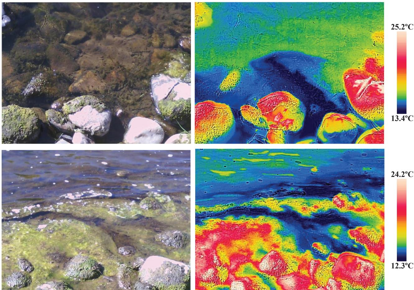
Figure A13.3. Visible light (left) and thermal infrared (right) photos of the groundwater seep at Site 13. Cool (blue, ~12-13°C) groundwater was observed discharging outward from the riverbank (top). Algae around the groundwater seep was warmer than the river and masked some of the cool groundwater discharging (bottom).
