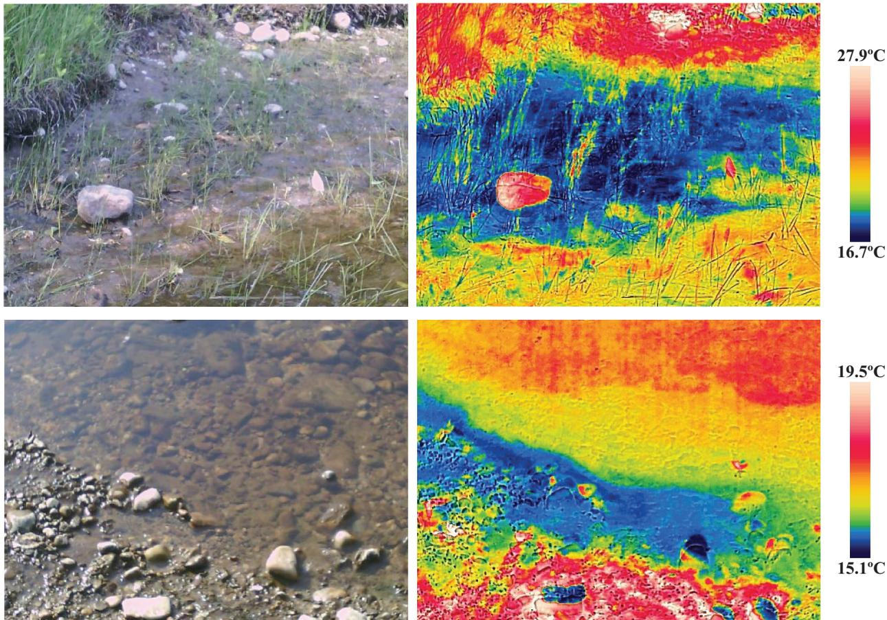
Figure A20.3. Visible light (left) and thermal infrared (right) photos of the groundwater seep at Site 20. Cool (blue, ~15-17°C) groundwater could be seen discharging from the saturated riverbank (top) and into the river (bottom).
