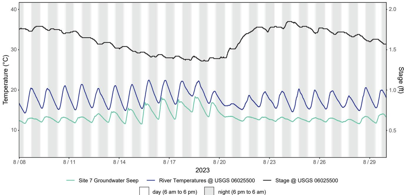
Figure A7.4. August 2023 logged temperatures at Site 7 groundwater seep (334292) compared to the river temperatures at the USGS gaging station Big Hole River near Melrose, MT (06025500). Diel groundwater temperature fluctuations were greater when stage was lower suggesting less flow at the monitored location when stage decreased.
