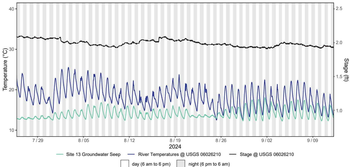
Figure A13.4. July–September 2024 logged temperatures at Site 13 groundwater seep (334298) compared to the river temperatures at the USGS gaging station Big Hole River near Glen, MT (06026210). Diel groundwater temperature fluctuations generally increased throughout the summer.
