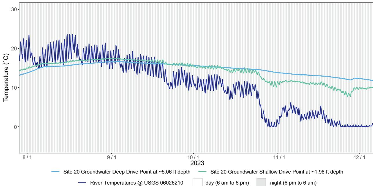
Figure A20.4. August-December 2023 logged temperatures at Site 20 groundwater seep. The groundwater seep (327512, 327511) is cooler than the river temperatures at the USGS gaging station Big Hole River near Glen, MT (06026210) during early August, but warmer than the river by mid-September. The deeper drive point has more consistent temperatures (less daily and annual fluctuations) compared to the shallow drive point that is more affected by heat transfer with the ground surface.
