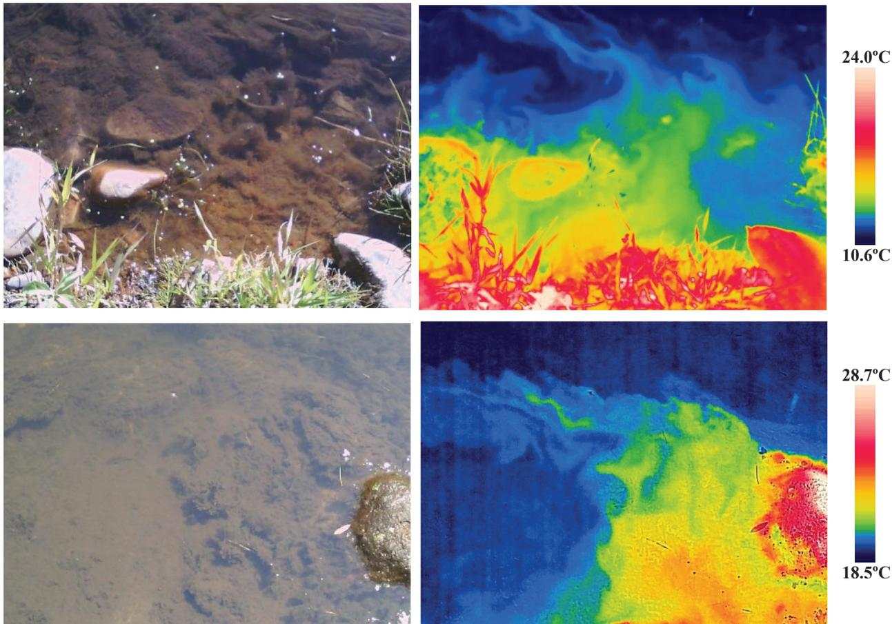
Figure A19.3. Visible light (left) and thermal infrared (right) photos of the seep at Site 19. This site often showed the water seeping from the riverbank to be slightly warmer (yellow, ~16-20°C) than the river.
