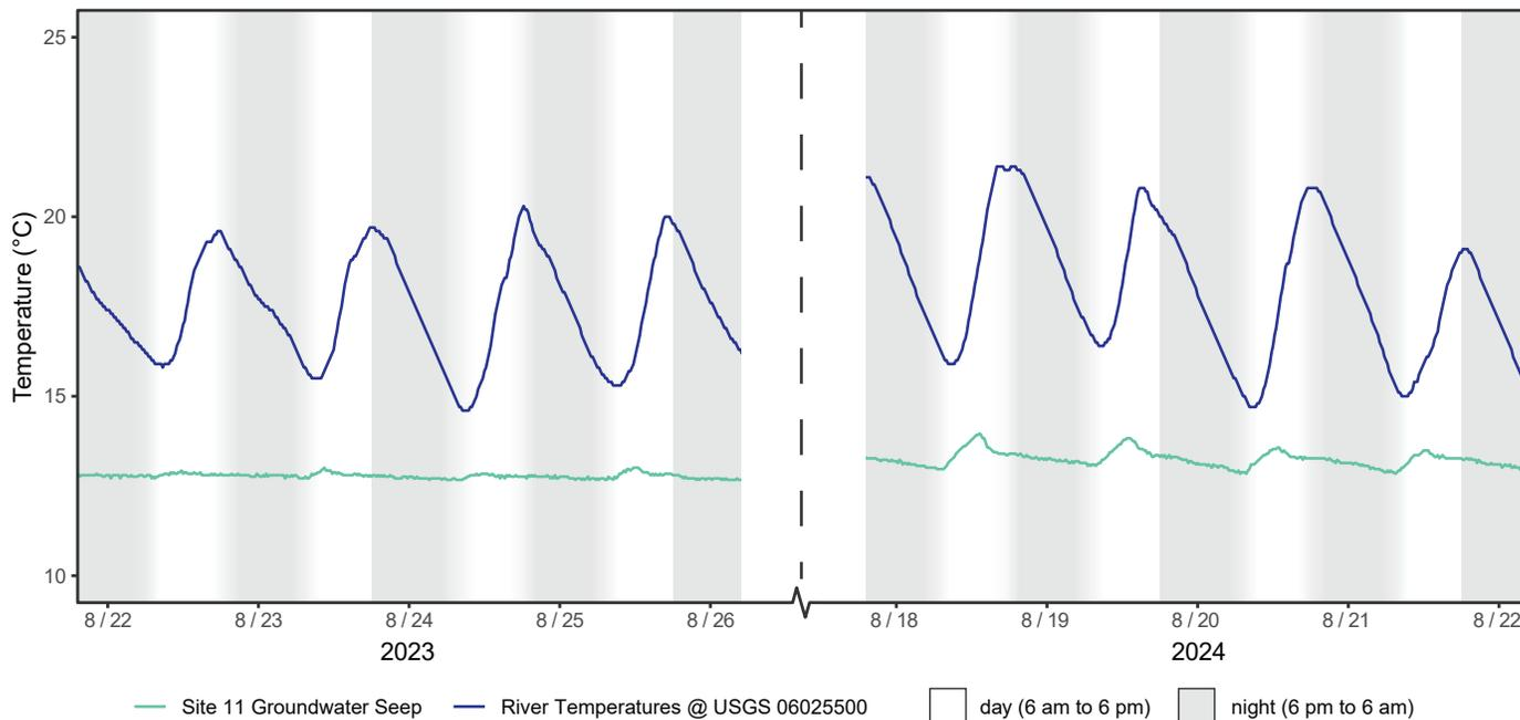
Figure A11.4. Comparison of August 2023 and 2024 logged temperatures at Site 11 groundwater seep (334296) compared to the river temperatures at the USGS gaging station Big Hole River near Melrose, MT (06025500). The groundwater seep temperatures remained steady around 13°C; diel fluctuations were smaller in 2023.
