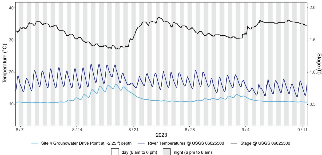
Figure A4.4. August-September 2023 logged temperatures at Site 4 groundwater seep (327516) compared to the river temperatures at the USGS gaging station Big Hole River near Melrose, MT (06025500). The groundwater temperatures at 2.25 ft depth in the drive point are cooler (~11°C) compared to the river (~15-21°C). Groundwater temperatures increased and diel groundwater temperature fluctuations were greater when river stage decreased.
