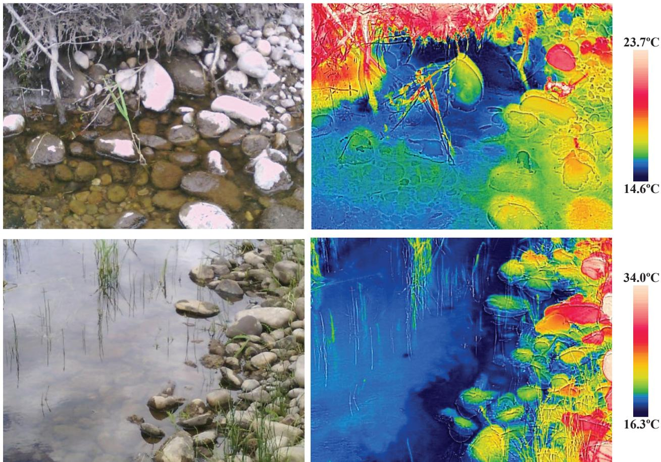
Figure A16.3. Visible light (left) and thermal infrared (right) photos of the groundwater seep at Site 16. This site commonly showed cool groundwater (dark blue, ~14-16°C) seeping from the edge and ponding. Sometimes it was discrete areas (top) and other times it was diffuse along the riverbank (bottom).
