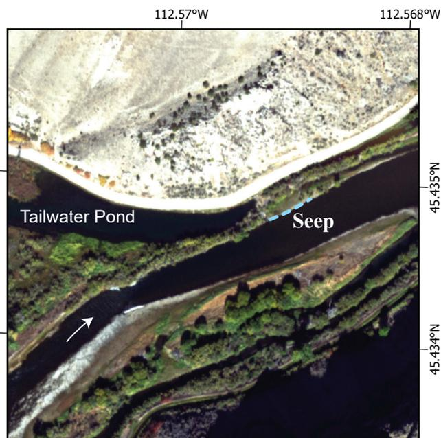
Figure A19.1. Aerial map of Site 19 showing the location of the seep (dashed blue line) derived from the tailwater pond.
