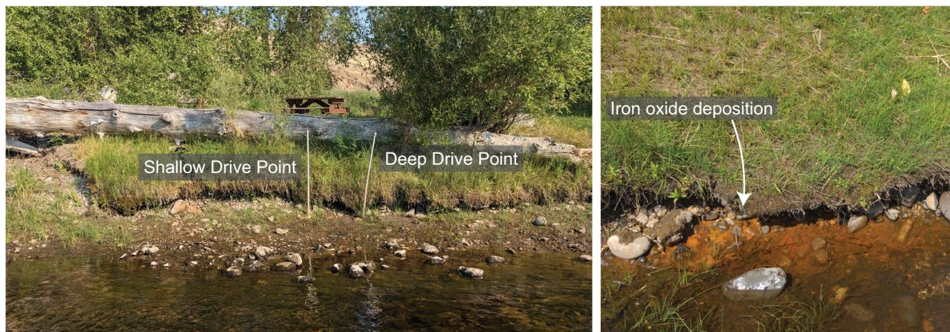
Figure A20.2. The shallow (~1.96 ft deep) and deep (~5.06 ft deep) drive points in the saturated riverbank of the groundwater seep (left). Iron-oxide deposition was commonly seen along the riverbank (right).
