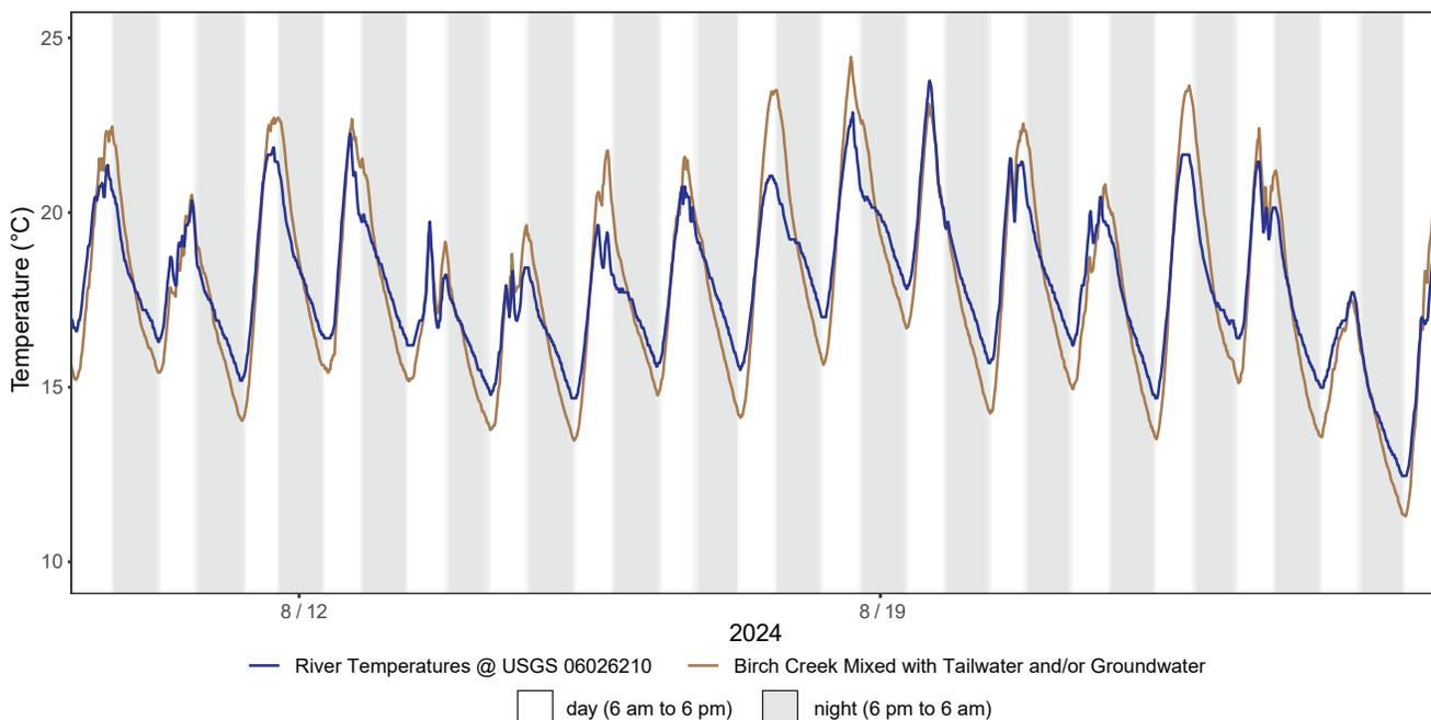
Figure B3.2. Mid- to late-August 2024 logged temperatures from Birch Creek (334307) compared to the river temperatures at the USGS gaging station Big Hole River near Glen, MT (06026210). The water from Birch Creek is generally warmer than the river during late afternoon and cooler than the river during early morning.
