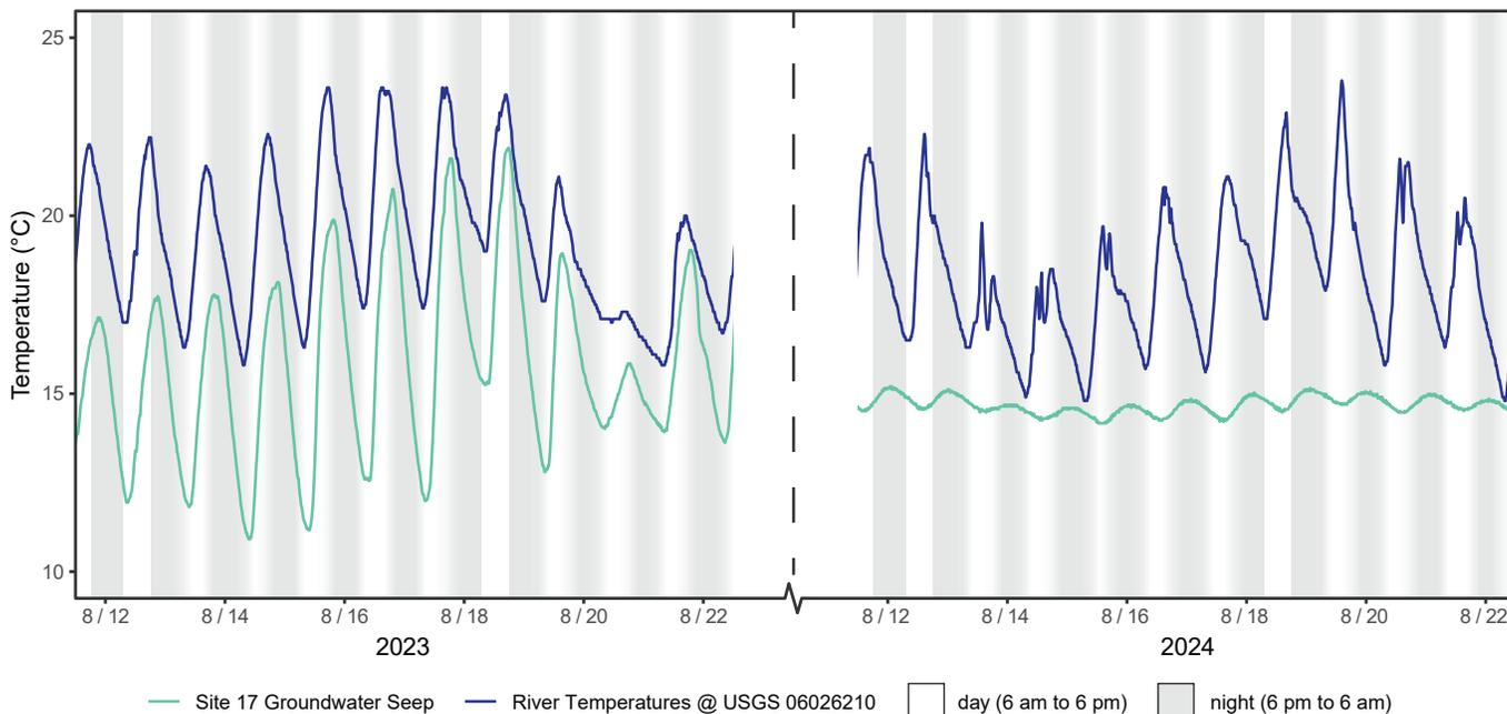
Figure A17.4. Comparison of August 2023 and 2024 logged temperatures at Site 17 groundwater seep (334302) compared to the river temperatures at the USGS gaging station Big Hole River near Glen, MT (06026210). Diel fluctuations of the groundwater seep changed between 2023 and 2024; this was likely due to where the groundwater seep was measured.
