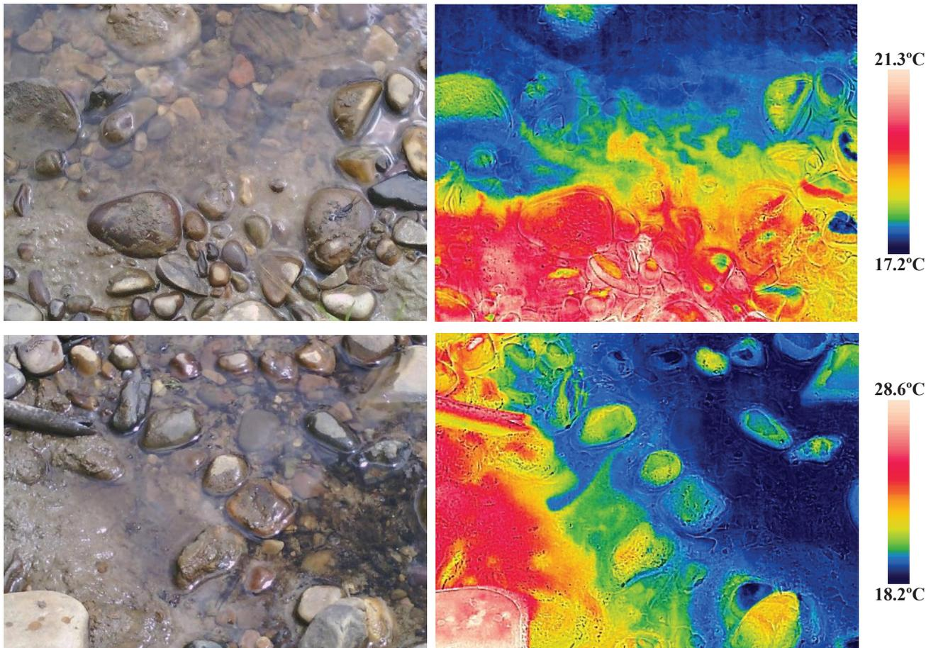
Figure A14.3. Visible light (left) and thermal infrared (right) photos of the groundwater seep at Site 14. The seep was often warmer (yellow, ~18-22°C) than the river.
