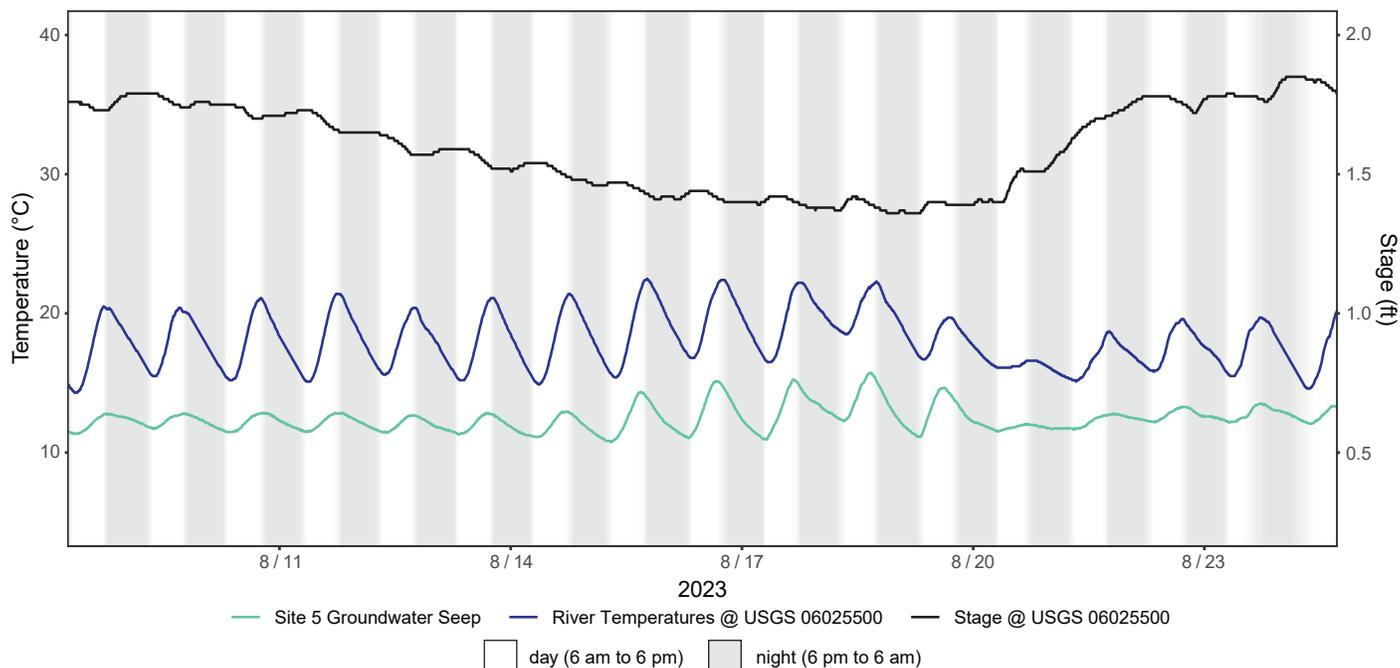
Figure A5.4. August 2023 logged temperatures at Site 5 groundwater seep (334290) compared to the river temperatures at the USGS gaging station Big Hole River near Melrose, MT (06025500). Diel groundwater temperature fluctuations were greater when stage was lower.
