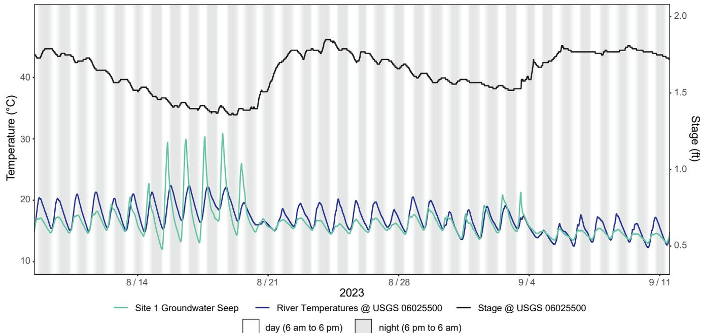
Figure A1.4. August–September 2023 logged temperatures at Site 1 groundwater seep (334283) compared to the river temperatures at the USGS gaging station Big Hole River near Melrose, MT (06025500). The minimum groundwater seep temperatures are similar to the river temperatures. Higher diel fluctuations occur when river stage was lower.
