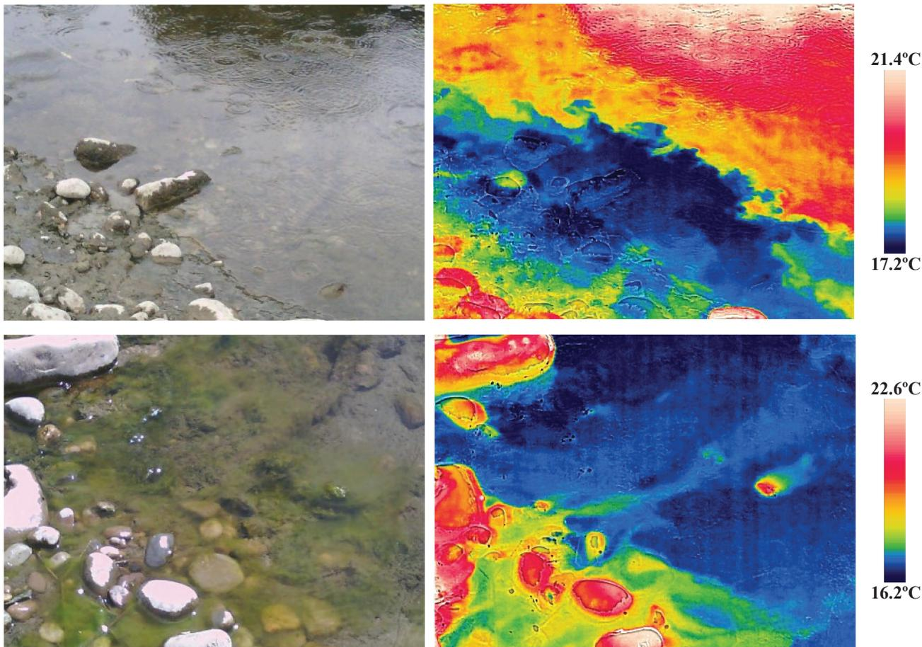
Figure A8.3. Visible light (left) and thermal infrared (right) photos of the hyporheic seep at Site 8. Depending on the river temperatures, the hyporheic water appeared cool (top; July 2024) or warm (bottom; August 2024) compared to the river temperatures. Algae was common near the hyporheic site during low flow (bottom left).
