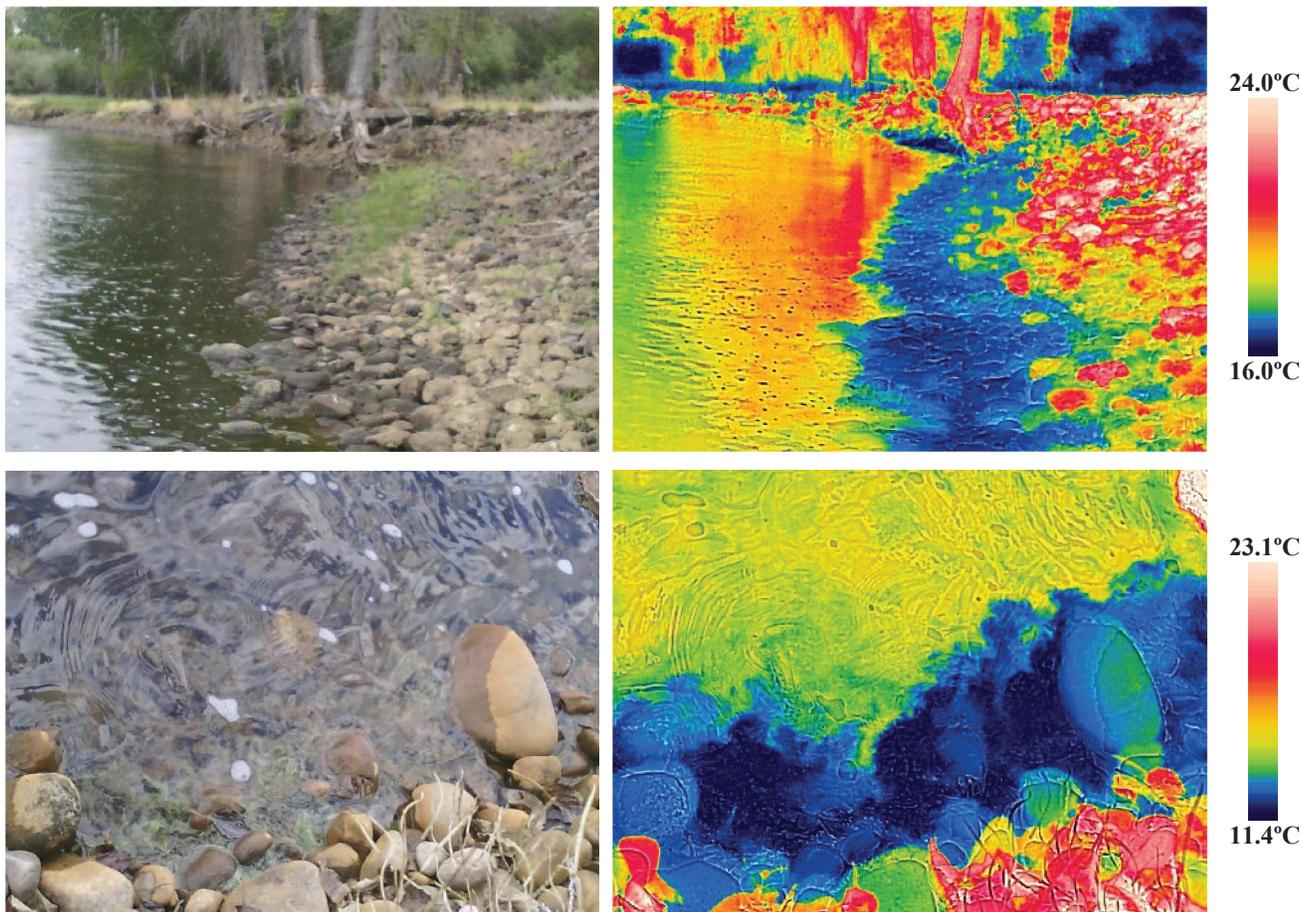
Figure A9.3. Visible light (left) and thermal infrared (right) photos of the groundwater seep at Site 9. Cool (blue, ~11-16°C) groundwater was observed discharging outward 2-4 ft from the cobble riverbank (top). A view from above the site showed the groundwater mixing with the river (bottom).
