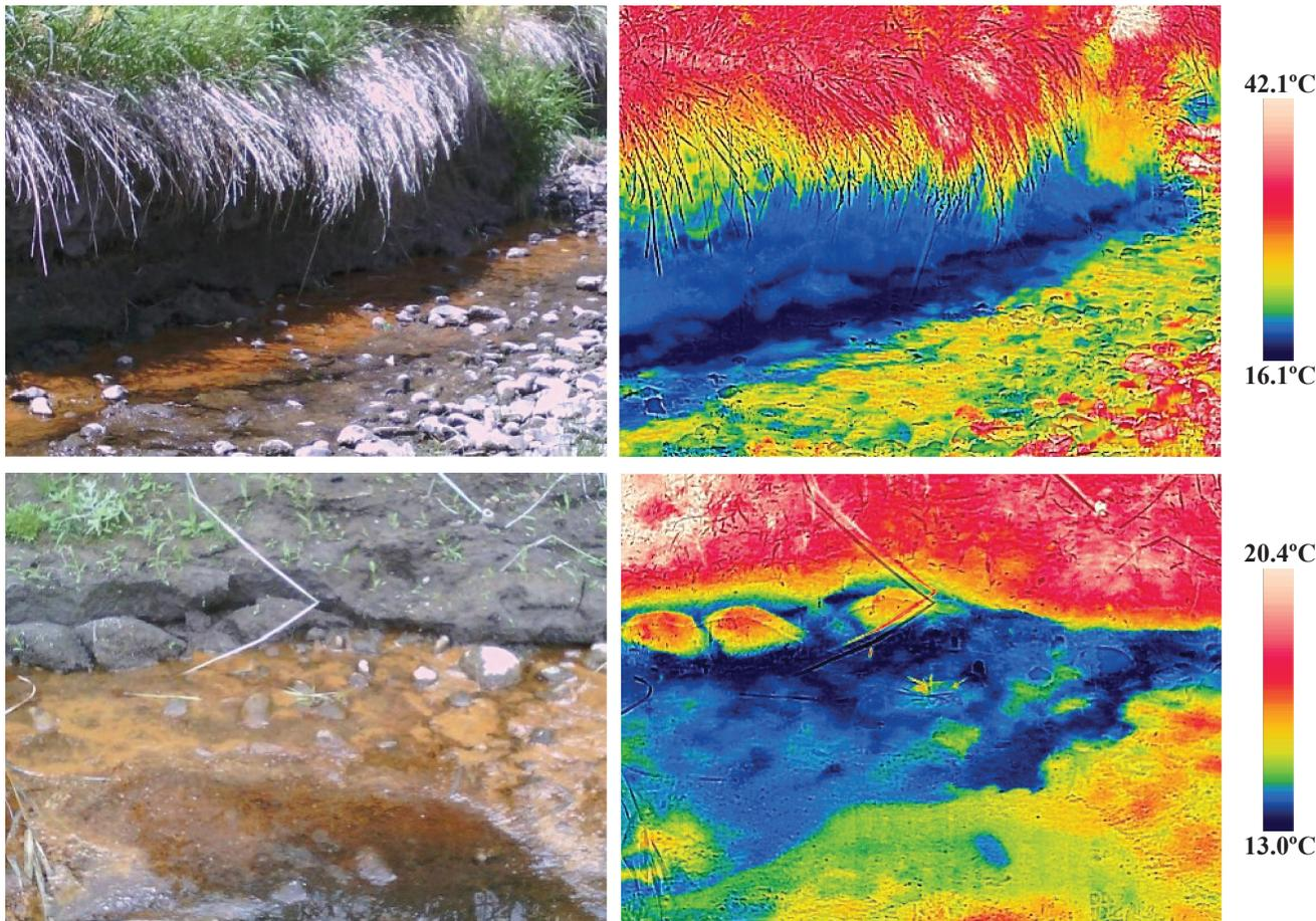
Figure A18.3. Visible light (left) and thermal infrared (right) photos of the groundwater seep at Site 18. This site commonly had cool groundwater (dark blue, ~13-16°C) seeping from the edge and ponding.
