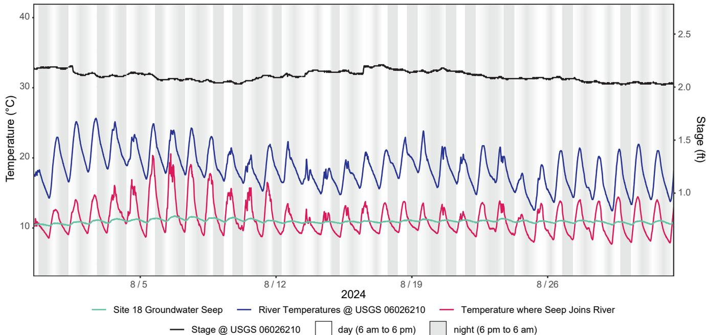
Figure A18.4. August 2024 logged temperatures at Site 18 groundwater seep (334303) compared to the river temperatures at the USGS gaging station Big Hole River near Glen, MT (06026210). Temperature was also monitored where the ponded groundwater reached the river (~200 ft away; 334338; see fig. A18.1). As the discharged groundwater flowed over the gravel bar it warmed as much as 10°C during midday.
