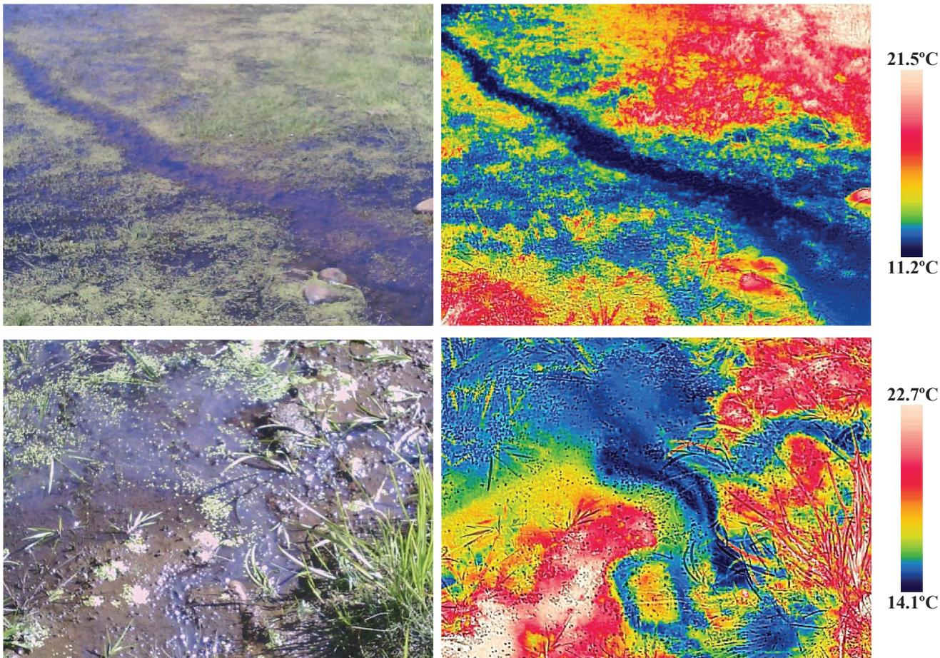
Figure A17.3. Visible light (left) and thermal infrared (right) photos of the groundwater seep at Site 17. Vegetation, which warmed in sunlight, often masked the thermal signal at this site (top). Discrete groundwater seeps could be seen on the edges of the ponded area (bottom).
