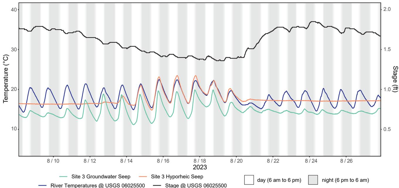
Figure A3.4. August 2023 logged temperatures at Site 3 groundwater seep (334288) and hyporheic seep (334289) compared to the river temperatures at the USGS gaging station Big Hole River near Melrose, MT (06025500). The hyporheic temperatures approximated average river temperatures while the groundwater seep temperatures were cooler than the river. Diel temperature fluctuations were greater when stage was lower suggesting less flow at the monitored spots.
