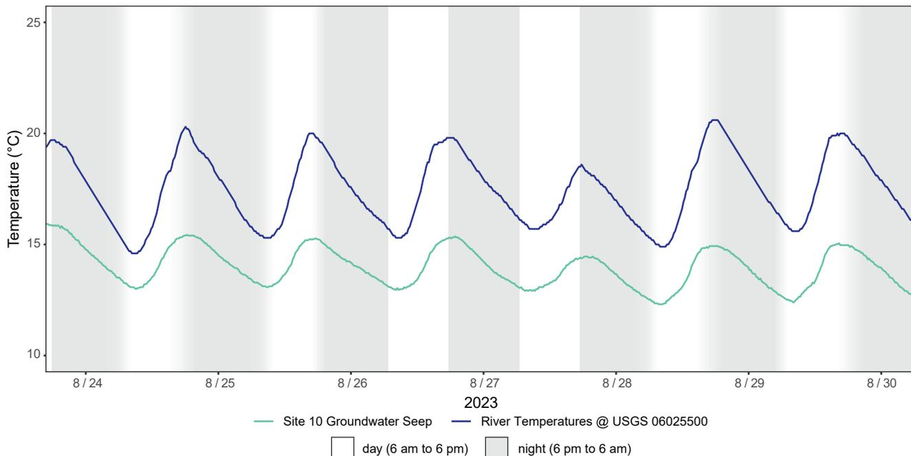
Figure A10.4. August 2023 logged temperatures at Site 10 groundwater seep (334295) compared to the river temperatures at the USGS gaging station Big Hole River near Melrose, MT (06025500). The groundwater temperatures were cooler than river temperatures. Diel groundwater fluctuations were ~2°C.
