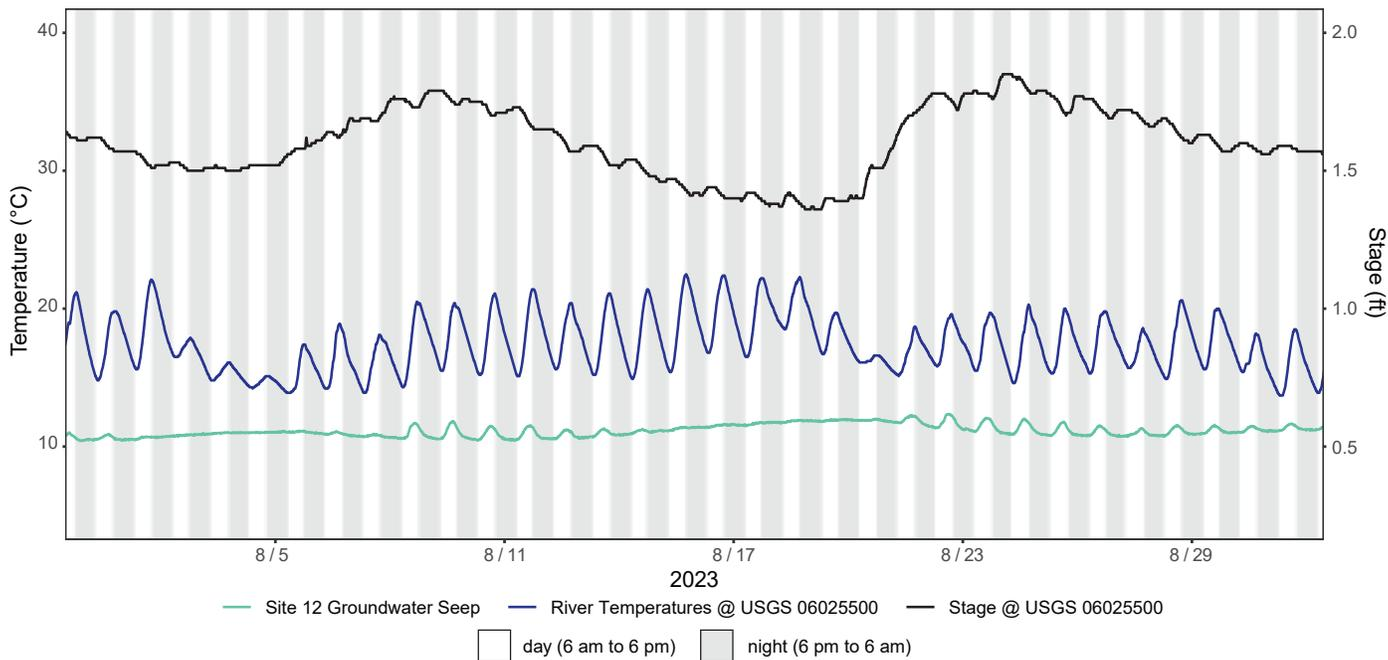
Figure A12.4. August 2023 logged temperatures at Site 12 groundwater seep (334297) compared to the river temperatures at the USGS gaging station Big Hole River near Melrose, MT (06025500). The groundwater seep showed greater diel fluctuations when the stage was higher (and likely the ponded area was also higher).
