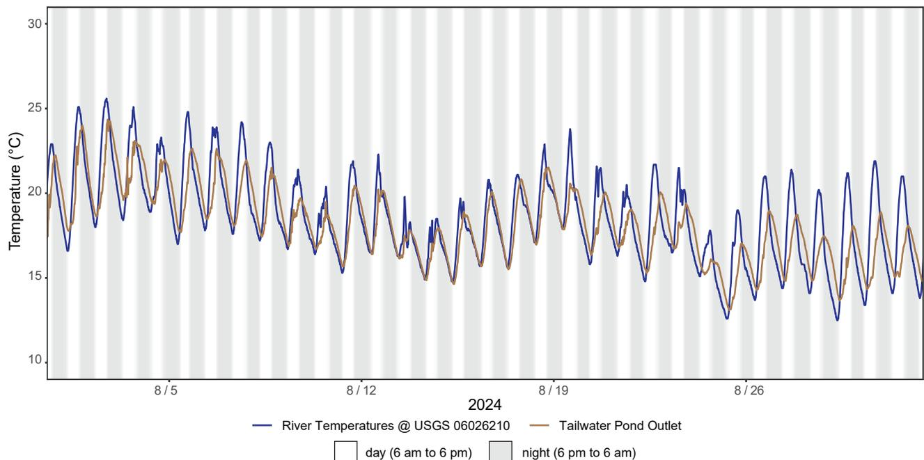
Figure B4.2. August 2024 logged temperatures from the southern tailwater (334308) compared to the river temperatures at the USGS gaging station Big Hole River near Glen, MT (06026210). The ponded tailwater had smaller diel fluctuations compared to the river and generally reached minimum and peak temperatures a couple hours later than the river.
