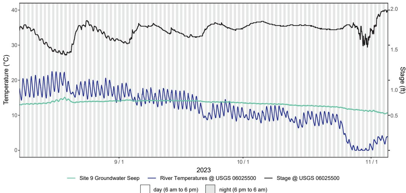
Figure A9.4. August-November 2023 logged temperatures at Site 9 groundwater seep (334294) compared to the river temperatures at the USGS gaging station Big Hole River near Melrose, MT (06025500). Groundwater temperatures were consistent at around 13-15°C; groundwater temperatures were cooler than the river during August and early September and warmer than the river in late September through November.
