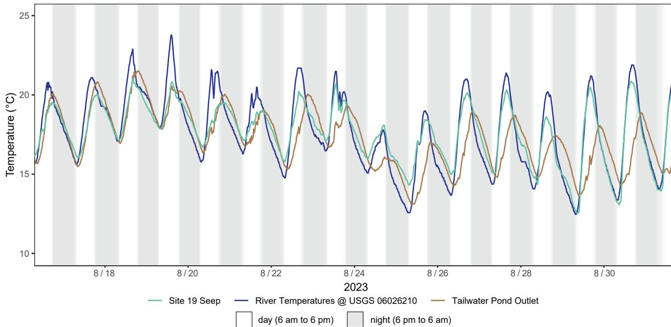
Figure A19.4. Late August 2023 logged temperatures at Site 19 seep (334304) compared to the river temperatures at the USGS gaging station Big Hole River near Glen, MT (06026210) and the adjacent tailwater pond outlet (334308) temperatures. The seep temperatures are more similar to the tailwater pond outlet from 8/17 to 8/22 and more similar to the river temperatures from 8/23 to 8/31, suggesting the amount of water seeping through the riverbank from the tailwater pond varied with time.
