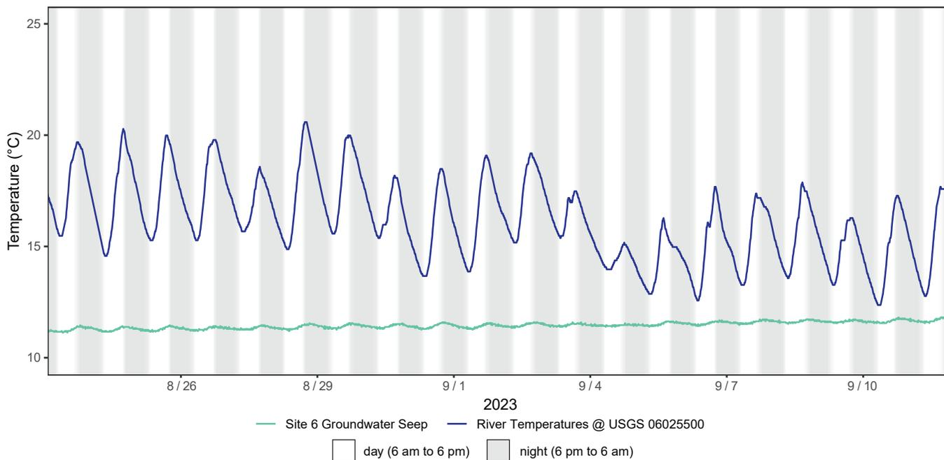
Figure A6.4. August-September 2023 logged temperatures at Site 6 groundwater seep (334291) compared to the river temperatures at the USGS gaging station Big Hole River near Melrose, MT (06025500). Groundwater temperatures were consistent around 11-12°C with generally small <0.5°C diel fluctuations compared to the ~5-6°C diel fluctuations of the river.
