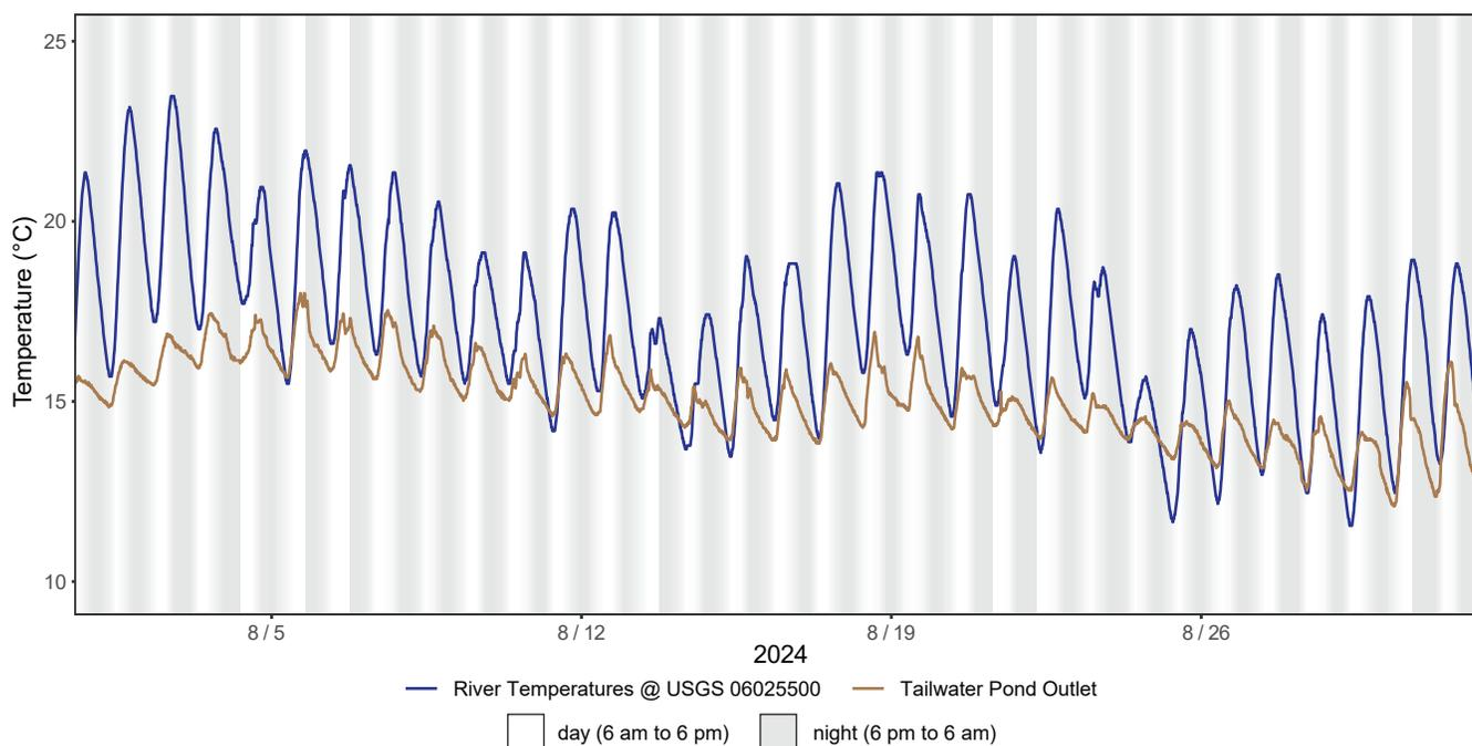
Figure B1.2. August 2024 logged temperatures from the northern tailwater return (334305) compared to the river temperatures at the USGS gaging station Big Hole River near Melrose, MT (06025500). The northern tailwater return was generally cooler (up to 7°C cooler) than the river except in the early morning.
