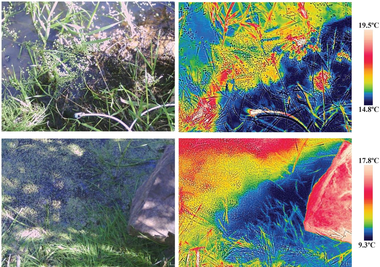
Figure A10.3. Visible light (left) and thermal infrared (right) photos of the groundwater seep at Site 10. Thermal contrast was only seen at the edges of the ponded water because the ponded water often became warm during the day.
