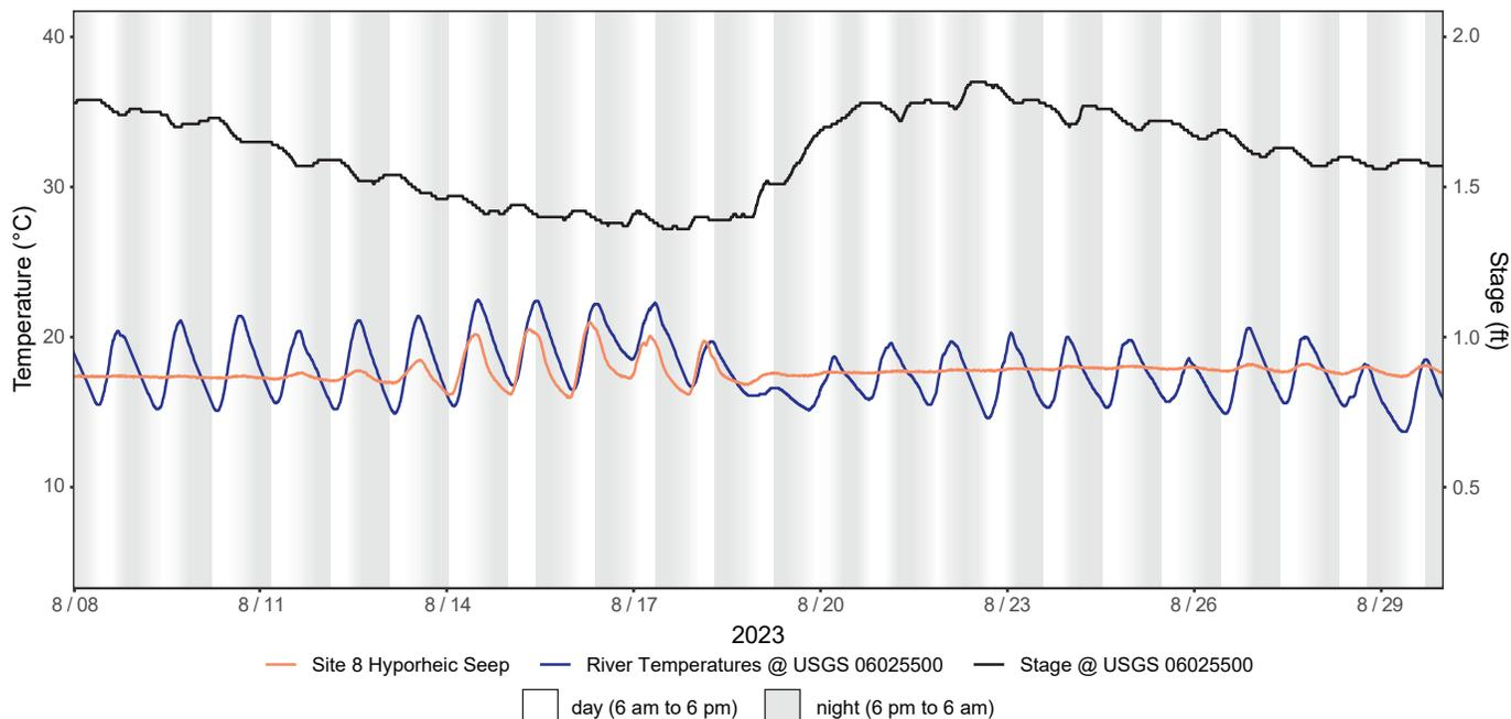
Figure A8.4. August 2023 logged temperatures at Site 8 hyporheic seep (334293) compared to the river temperatures at the USGS gaging station Big Hole River near Melrose, MT (06025500). The hyporheic temperatures were approximately the average of river temperatures. Diel hyporheic temperature fluctuations were greater when stage was lower.
