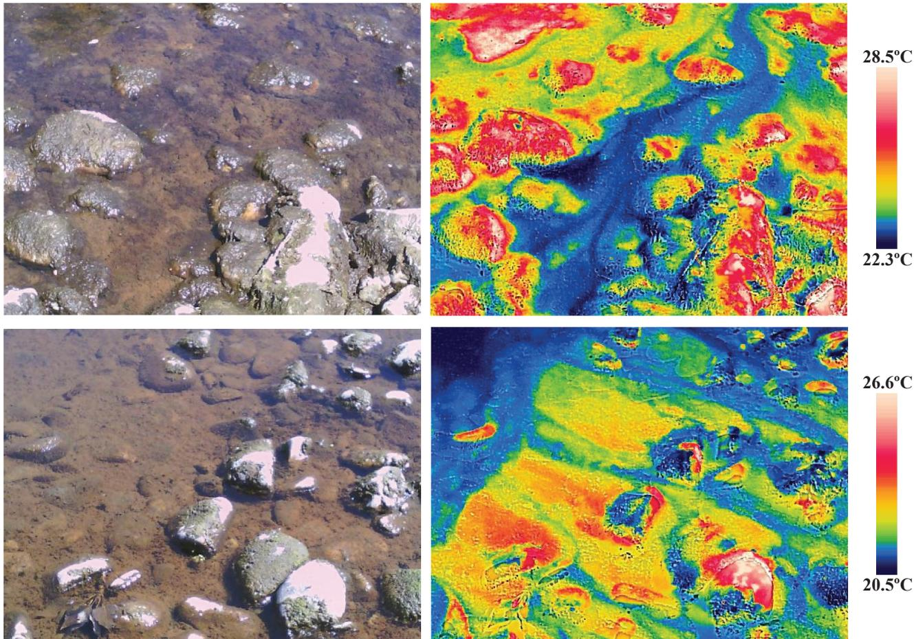
Figure A15.3. Visible light (left) and thermal infrared (right) photos of the groundwater seep at Site 15. This site was shallow and heated up during the day. Groundwater appeared cooler than the surroundings, but was warm (20–22°C) compared to other groundwater sites.
