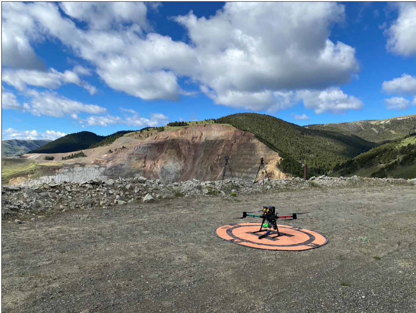
Figure 3-15. Montana Tunnels: UAV equipped with Data Sonde.
