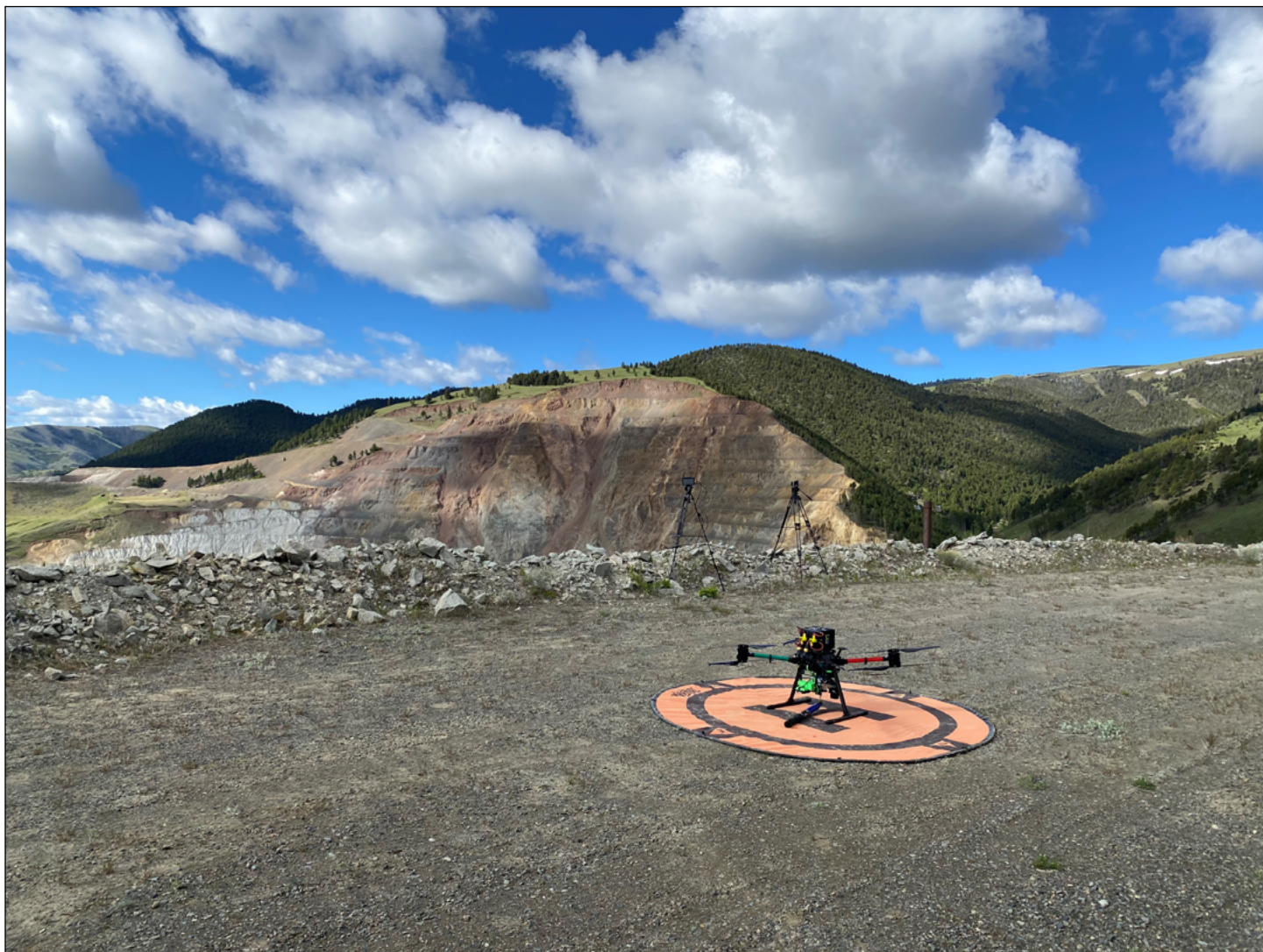
Figure 3-15. Montana Tunnels: UAV equipped with Data Sonde.
