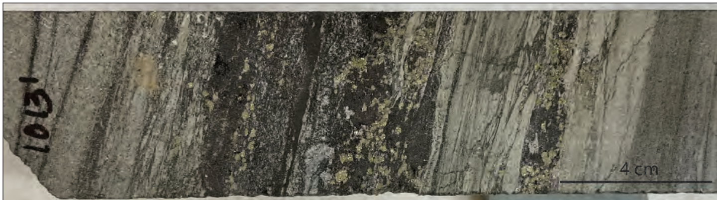
Figure 5. Drill core from Ruby zone showing weakly sheared, magnetite-matrix breccias with pyrite in quartz-rich siltite (Sample IC22-02-1013).
