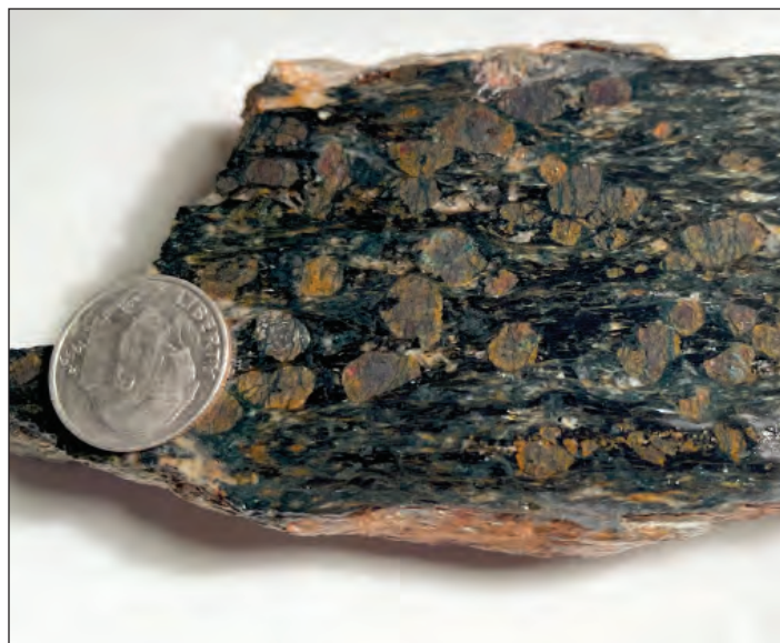
Figure 9. Hand sample of garnet-biotite schist from the Salmon Canyon copper prospect. Garnet-rich samples from the prospect commonly contain interstitial metal-sulfides. Garnets are rimmed by chlorite, indicating late-stage disequilibria with biotite.
