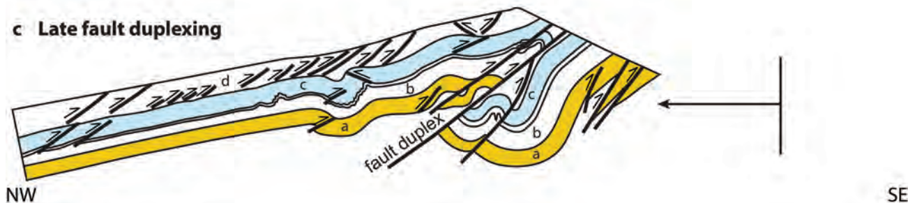
Figure 18. Balanced and restored cross-section of Kiorpes (1990). In each time step, shortening is shown as an arrow. Dashed lines show trajectory of future thrusts. Colors and unit labels correspond to those in the previous figure.
