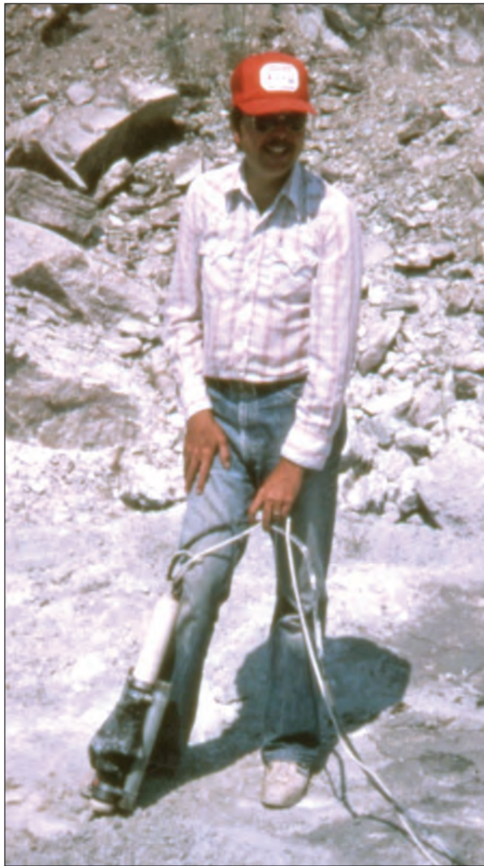
Figure 4. Deploying the downhole geophone. The black hose contained the geophone signal wires and the pneumatic tube for inflating the packing bladder, the black bulge at the base of the tool. The “drawworks” was the student or me manually handling the white polyethylene rope, which stretched under the weight of the tool and the hose, leading to uncertainty in the exact depth at which a reading was made. Photo by James Buice.
