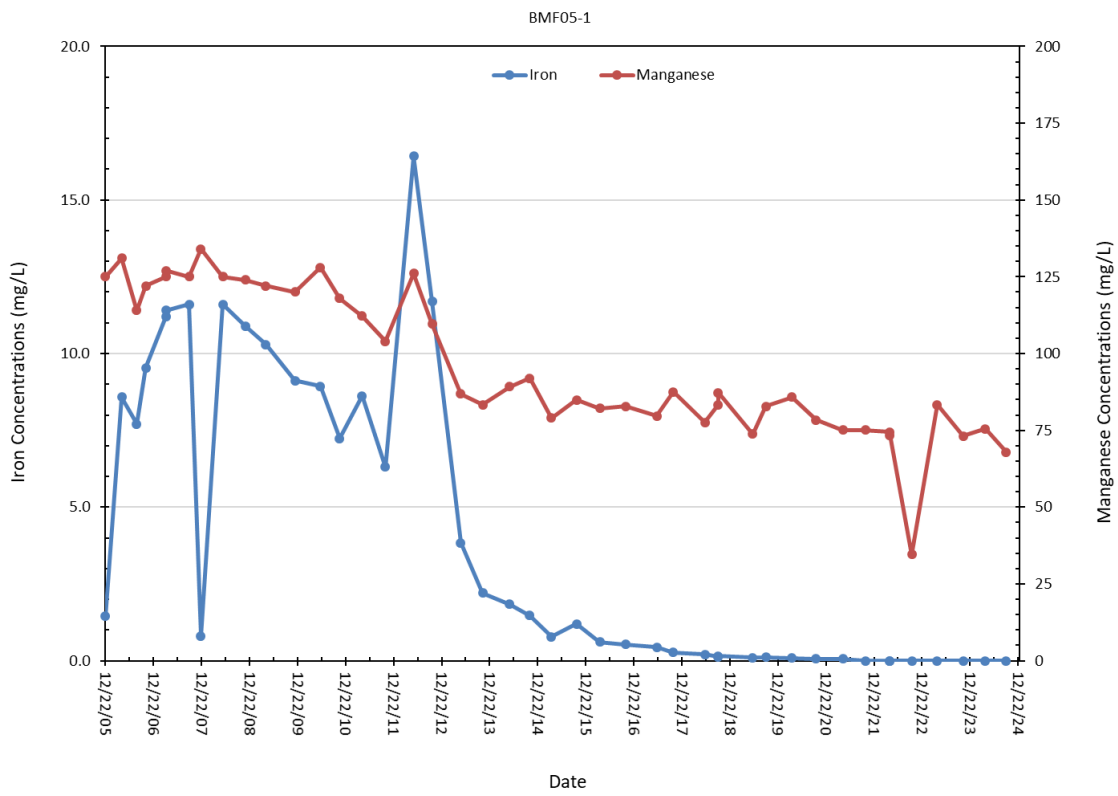
Figure 2-26. Iron and manganese concentration trends in well BMF05-1.
