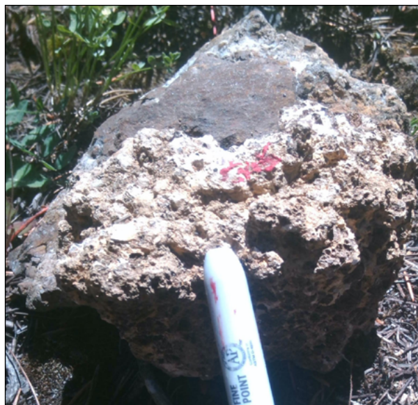
Figure 3. A sample of oxidized Au-Bi ore with 4 g/t Au and 1.25 wt.% Bi from a historic mine dump in Powell County, Montana. Photo by Adrian Van Rythoven, MBMG.
