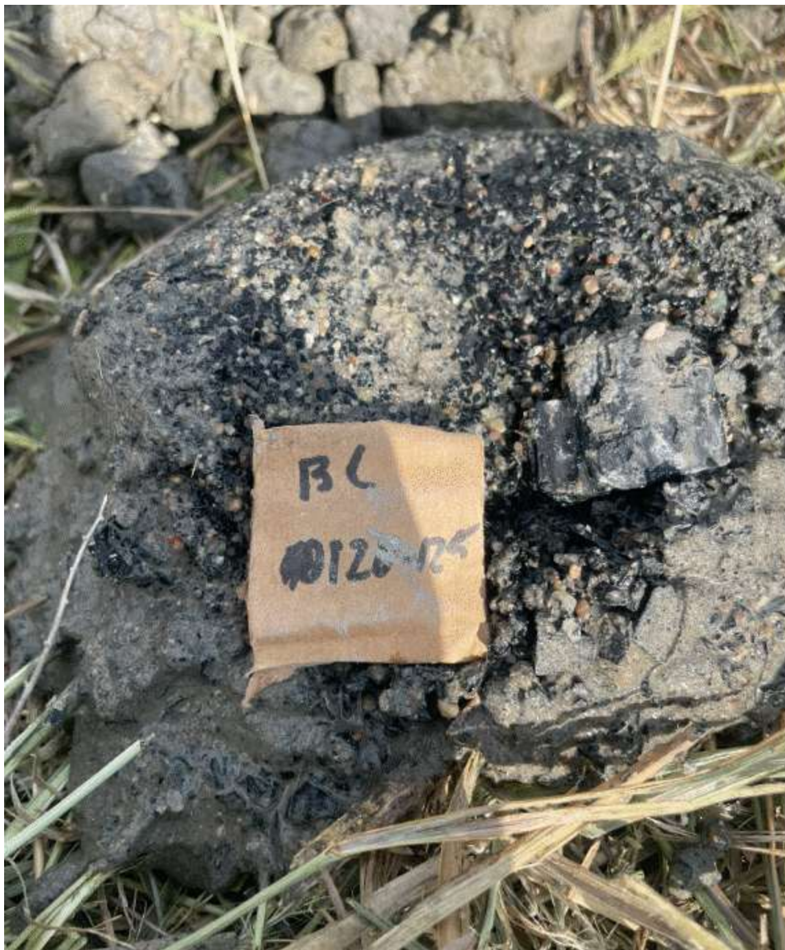
Figure A7. Cuttings from the Big Muddy well (MNMG-338719) showing the sand and gravel just above the Fort Union Formation.
