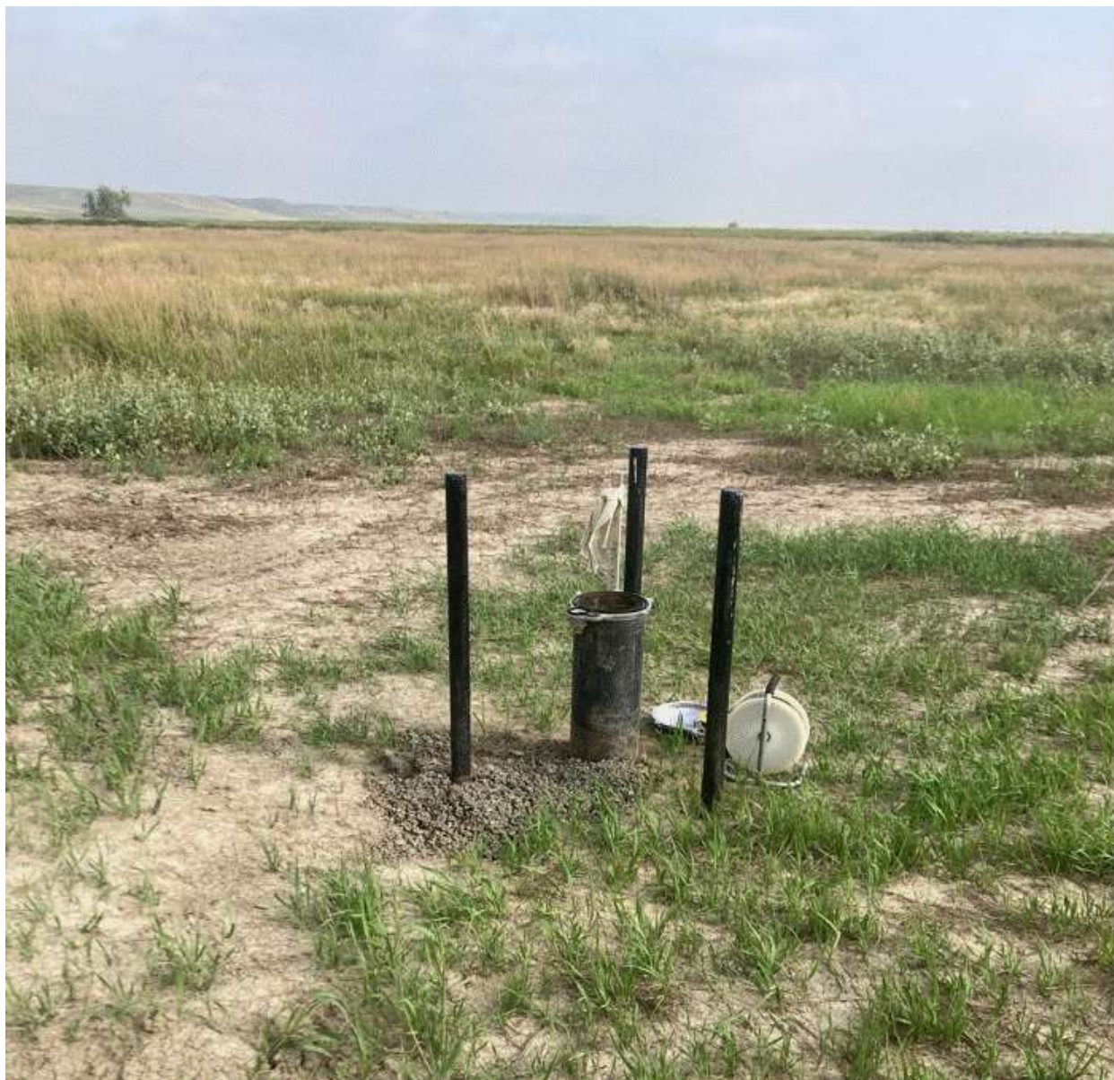
Figure A4. Bollards were installed around the MBMG—Big Muddy well ( MBMG-338719).
