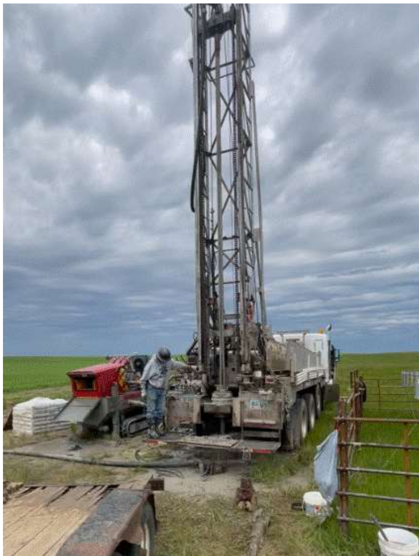
Figure A1. Wells were drilled with a mud rotary rig.
