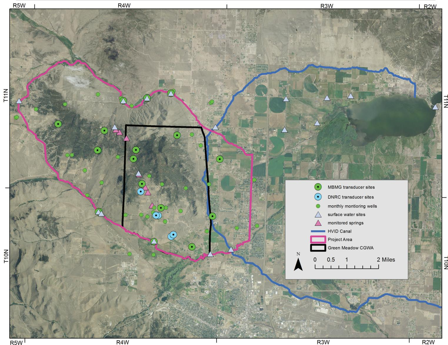
Figure 8. A monitoring network of 67 wells, 7 springs, and 18 surface-water sites provided the Scratchgravel Hills Groundwater Investigation's observational basis. Note that the symbols for some sites are stacked.
