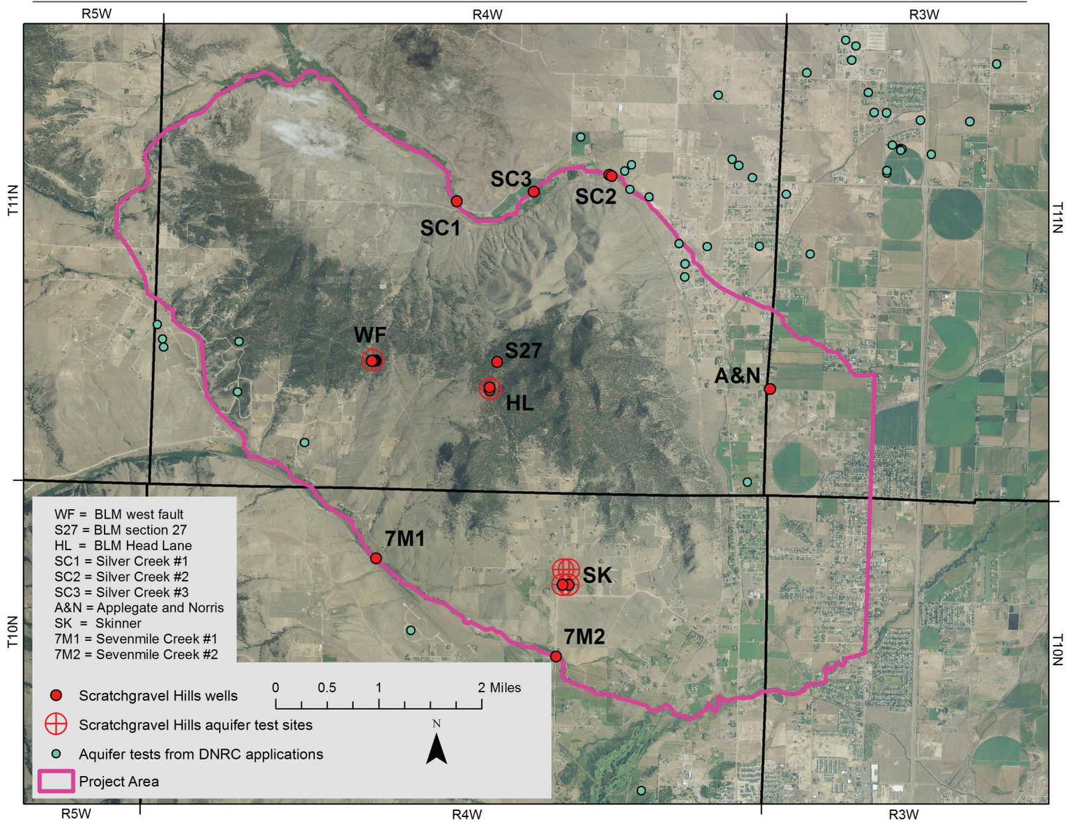
Figure 7. Wells were installed at 10 locations within the Scratchgravel Hills study area to acquire water-level information and to evaluate aquifer properties. Six aquifer tests were conducted. Aquifer test data from numerous DNRC water-rights applications also provided information on aquifer properties.
