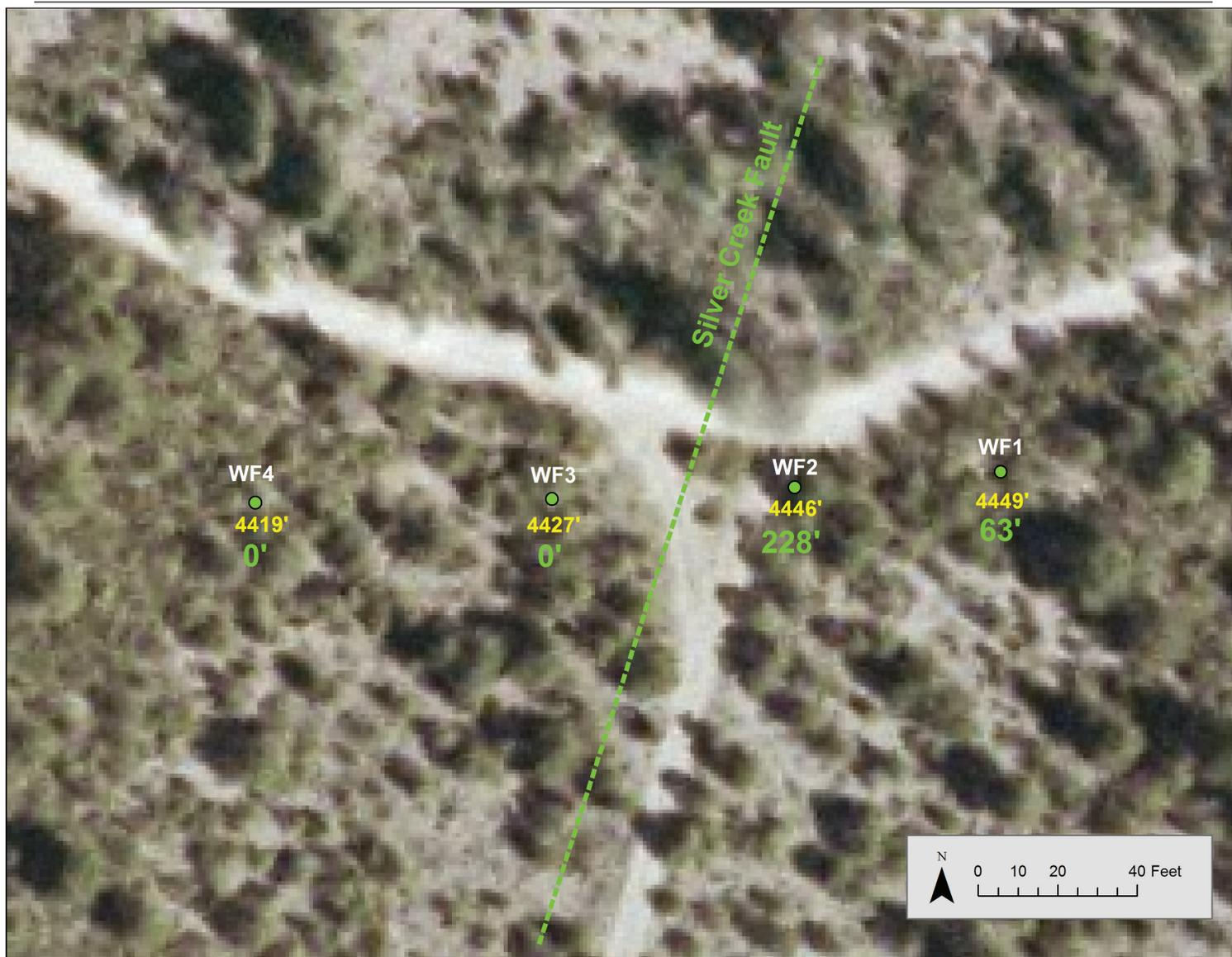
Figure 12. The West Fault Aquifer Test site in T. 11 N., R. 4 W., sec. 28 SWSW, transects the Silver Creek Fault. Static groundwater-level altitudes from November 9, 2010 (ft-amsl, in yellow) show an abrupt water-level difference of about 20 ft from east to west across the fault. A 24-hour pumping test at Well WF2 produced the maximum drawdowns (ft) shown in green.
