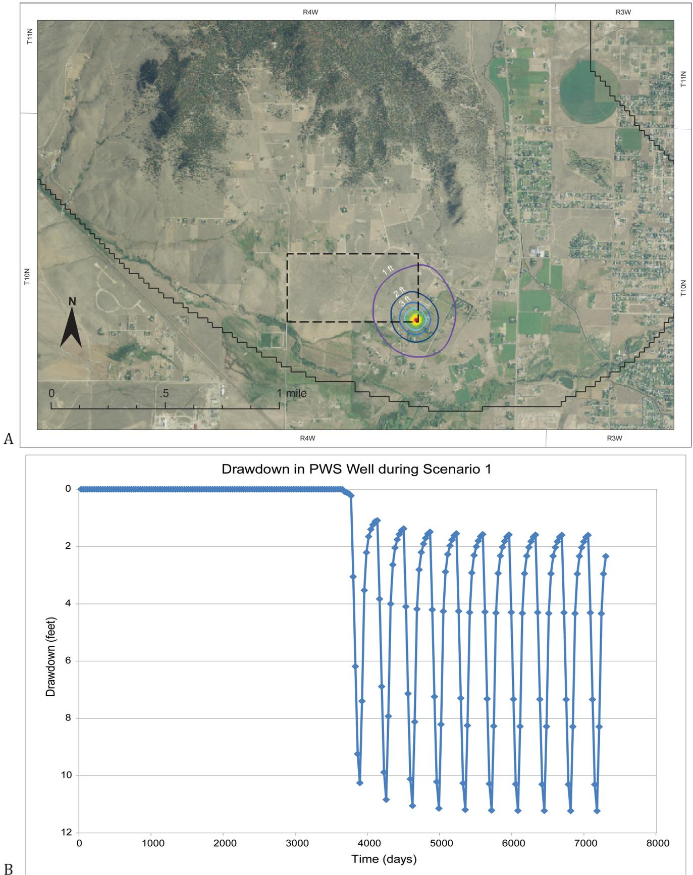
Figure 24. Scenario 1 illustrates modeled drawdown from a public water supply well located in the SE $\frac{1}{4}$ SE $\frac{1}{4}$ NE $\frac{1}{4}$  sec. 11, T. 10 N., R. 4 W., designed to provide water to 33 homes on 10-acre lots. This well is completed in the alluvium. The well's maximum radius of influence extends about 0.5 mile (A), its maximum drawdown is approximately 11 ft, and water levels stabilize during the 10-yr model run (B).
