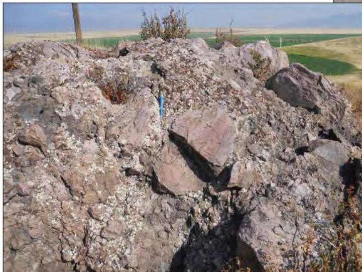
Figure 22. These photographs show the three main aquifers in the study area. Note the fine-grained nature of the Tertiary sediments. Secondary porosity in the volcanic rock makes this the most prolific aquifer in the study area.
