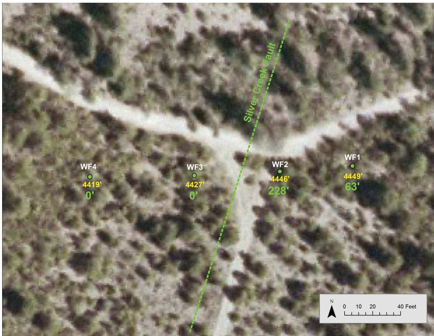
Figure 13. This well-installation site is located on the Silver Creek Fault. Static groundwater elevations from November 9th, 2010 (ftmsl, in yellow) showed an abrupt water-level change across the fault. A 24-hour pumping test was conducted at this site, and resulting drawdowns (ft) are shown in green. This site is located in T. 11 N., R. 4 W., sec. 28 SWSW. WF2 (well 257370) is at 46.6774301° N, 112.1230996° W.
