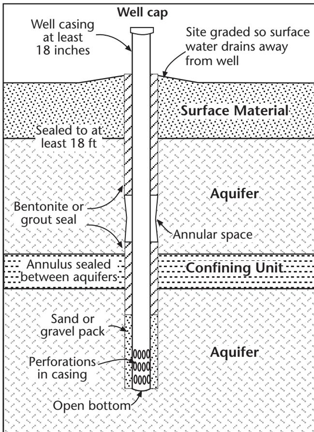
Figure G-8. Properly constructed wells are completed in single aquifers. In order to protect groundwater quality and maintain artesian pressures, wells should not serve as conduits from the surface to groundwater or connect separate aquifers.
