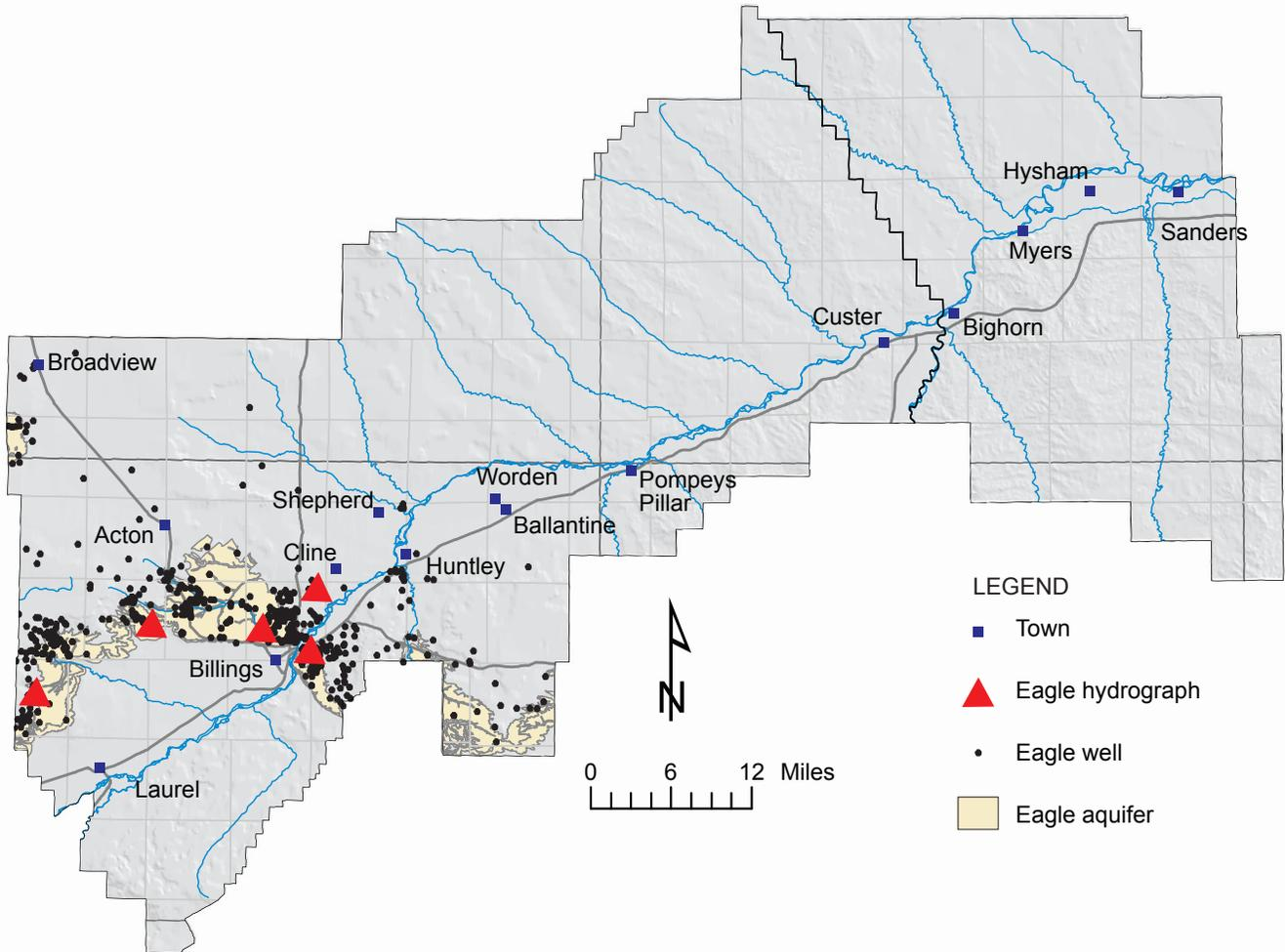
Figure 24. Water wells completed in the Eagle aquifer are concentrated in the greater Billings-to-Laurel areas, near to, and down dip from, the outcrop areas of the Eagle.
