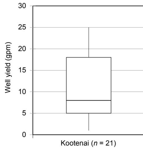
Figure 39. Reported well yields for the Kootenai aquifer average about 8 gpm.
