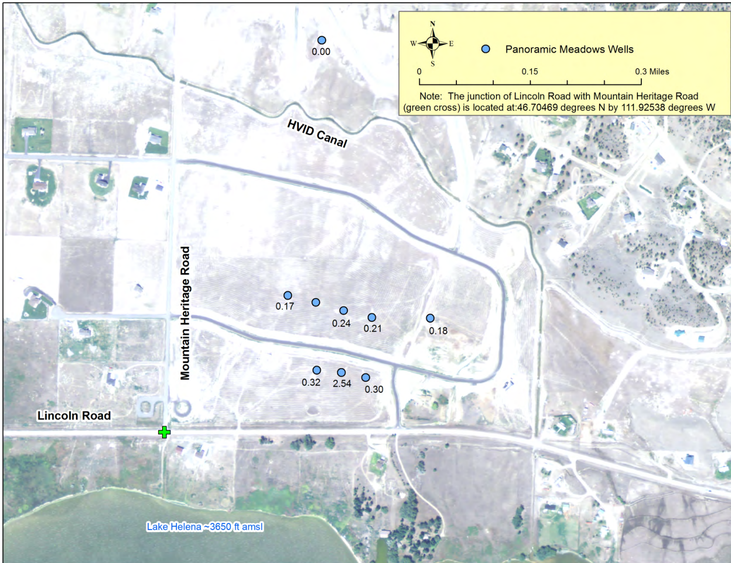
Figure PM18. Maximum drawdown (ft) observed during the Panoramic Meadows Aquifer test.
