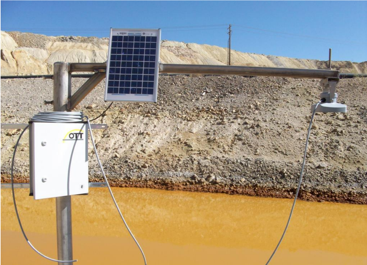
Figure 2-46. Radar system installation at the Horseshoe Bend weir monitoring station.
