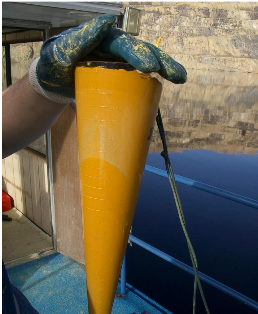
Figure 2-53. Accumulation of secondary iron precipitates in a sediment trap deployed in the Berkeley Pit for 150 days.
