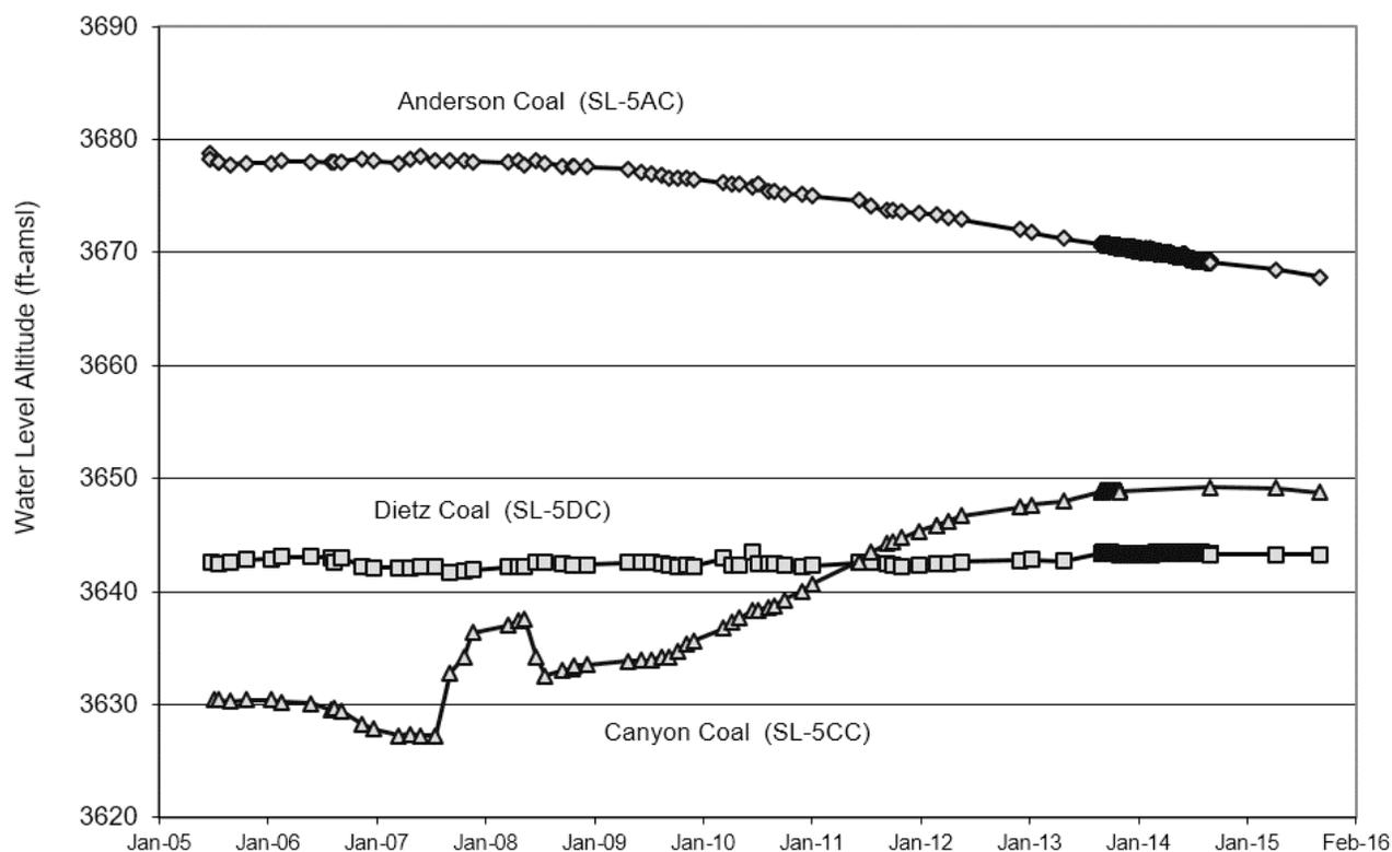
Figure 23. The increasing water level in the Canyon and decreasing water level in the Anderson may be a result of a failed seal in the neat cement in the Canyon coal well causing communication along the well bore. Alternatively, it may be that a nearby well has allowed the two aquifers to communicate.
