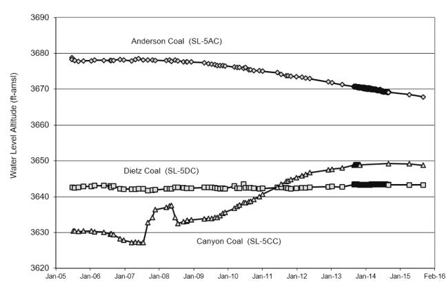
Figure 23. The increasing water level in the Canyon and decreasing water level in the Anderson may be a result of a failed seal in the neat cement in the Canyon coal well causing communication along the well bore. Alternatively, it may be that a nearby well has allowed the two aquifers to communicate.
