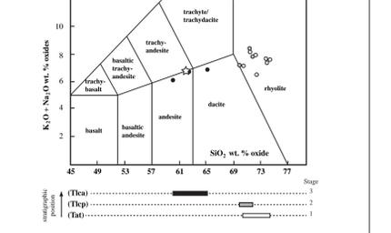
Figure 3. Rock type diagram shows the composition of Lowland Creek Volcanics samples collected in the Opportunity 7.5' quadrangle, after LeBas and others (1986). The star represents sample 93-15, analyzed by Dudas and others (2010). Note that this sample shows compositional zoning of the deposits to lower silica content with time.
