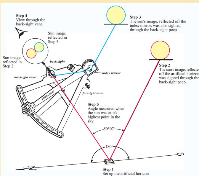
Taking a noon observation with octant and artificial horizon by the "back" method:
