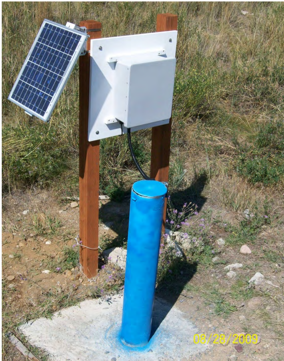
Figure 4.2-7. Telemetry system installed at well MW-213.
