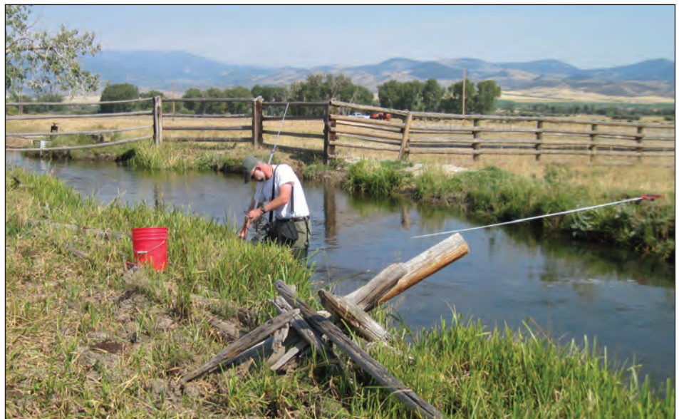
Figure 1. Canal flows were measured so that canal leakage rates could be calculated. Canal leakage is an important source of groundwater recharge in the Boulder River Valley.
