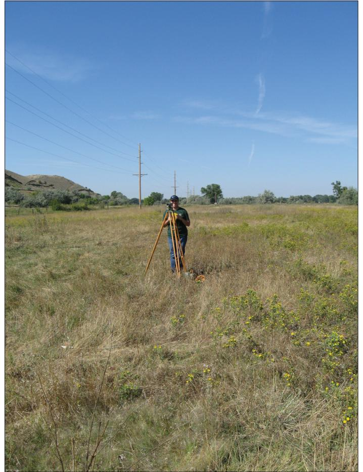
Figure A3-8b. Surveying relative well altitudes.
