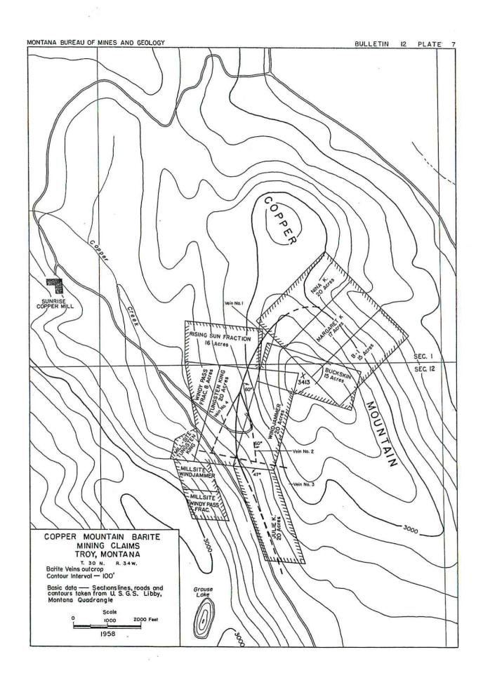
The property is developed by one 80-foot adit (assessible) on Vein No. 1, and a 35-foot adit on Vein No. 3, and several pits and cuts on the other veins.
