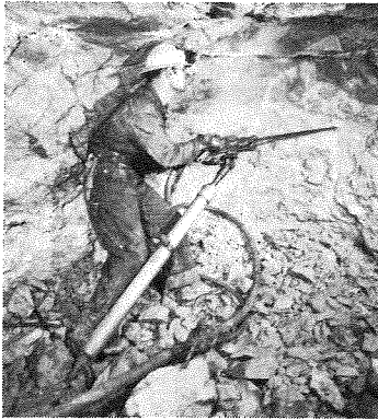
A. Air operated rock drill. (Courtesy Archibald Co.)
