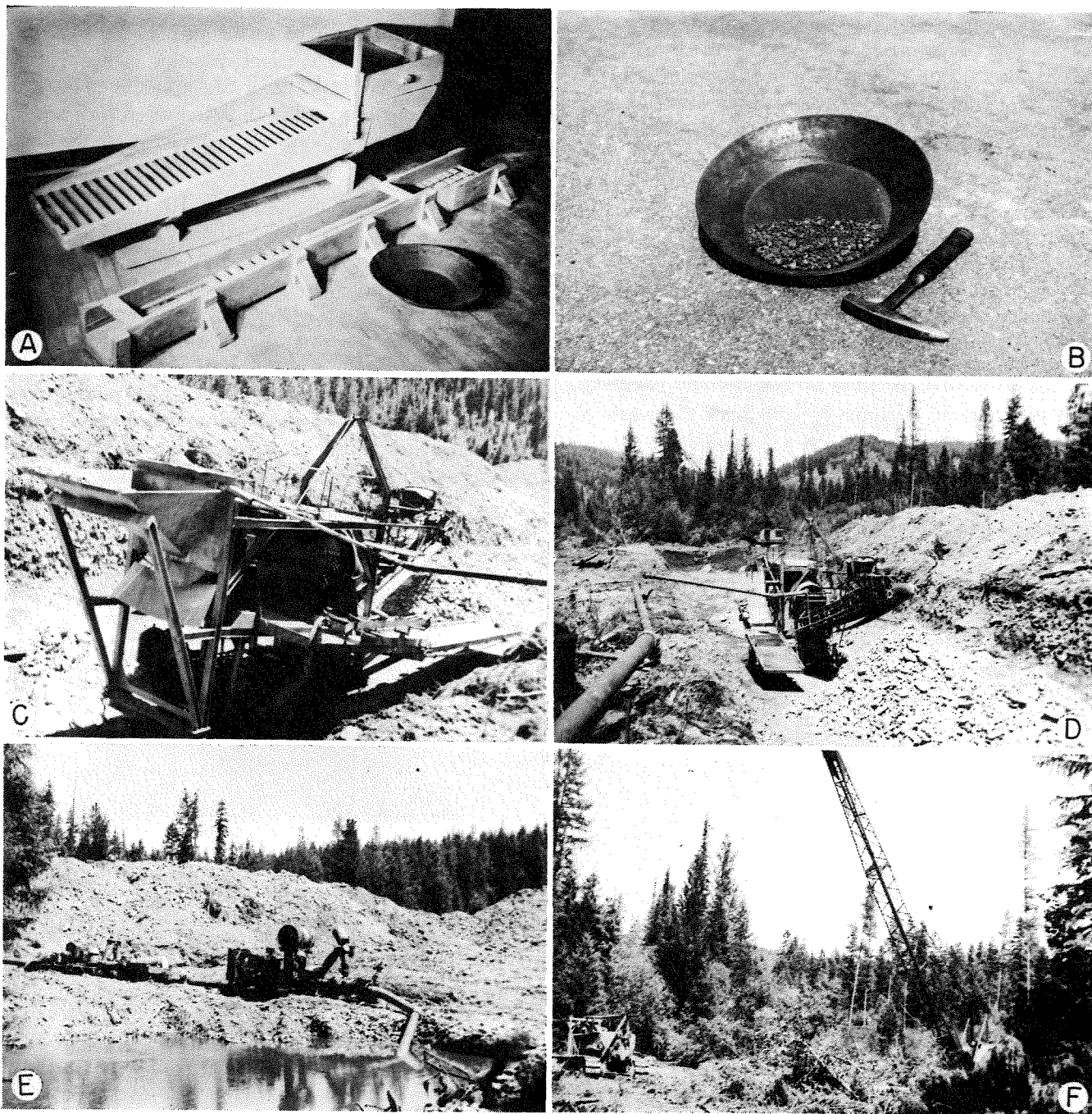
A. Rocker, in background, sluice box with various styles of riffles, in middle, and gold pan, in front. B. Gold pan partly filled with gravel. C. Side view of a dry-land dredge or gold-washing outfit. Loading hopper on left, rotating screen in middle, and sluice on lower right. D. The same washing plant viewed from the rear. E. Pump and pond that supply water to the washing plant. F. Clearing brush and stripping overburden preparatory to mining.
