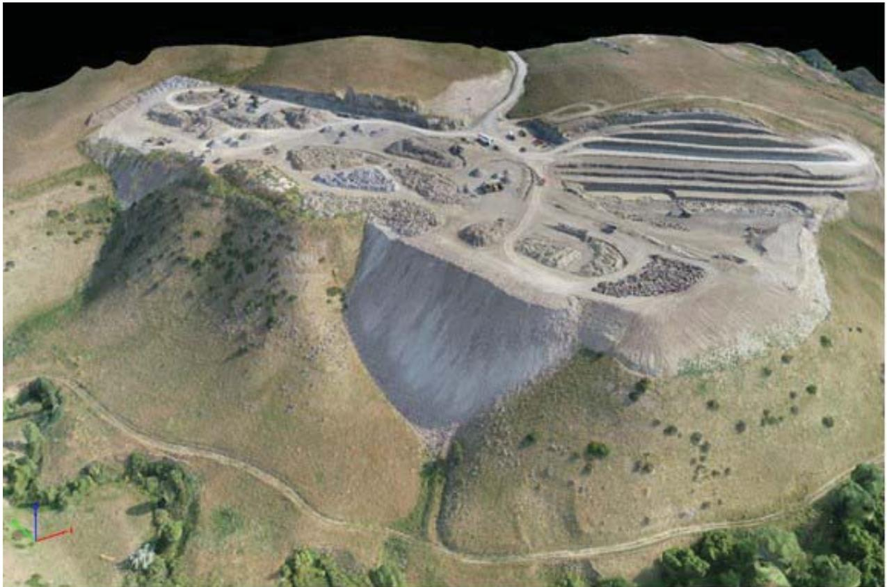
Figure 3. Three-dimensional stone site model rendered by Pix4Dmapper from aerial imagery collected on site with UAV.
