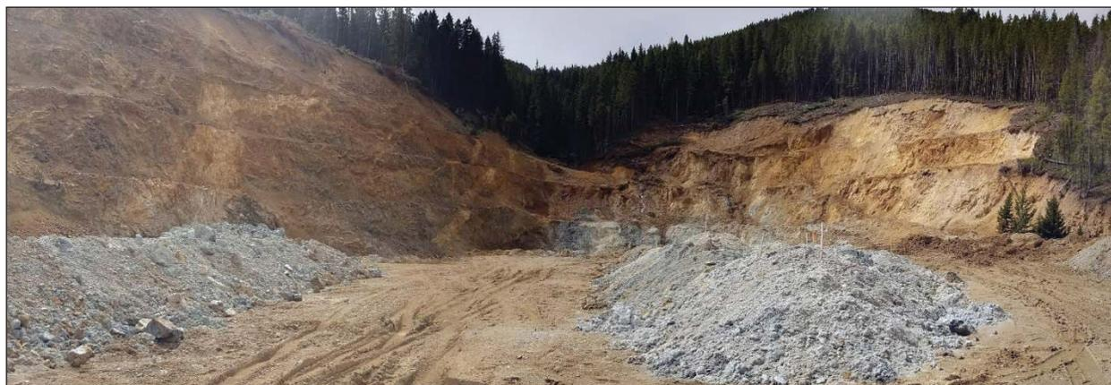
Figure 2. The Pacific Mine Pit, looking south (June 9, 2017, photo taken by Jon Rice). Note the east-dipping granite-pegmatite dikes and sills exposed in the east wall (left side of photograph), and the crumbly, oxidized schist exposed in the west wall. Hand samples were collected from the “high grade stockpile” in the foreground, on the left side of the photograph.
