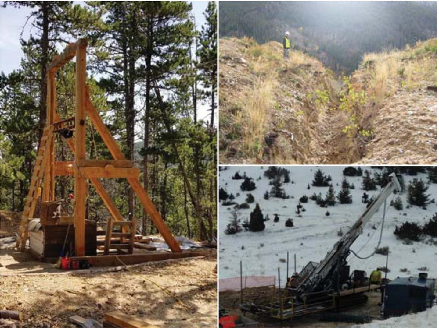
Figure 2. Examples of active exploration projects in Montana. Clockwise from top right: An exploration trench; a core drilling operation; a modern headframe built to access and remove samples from an historic underground shaft.
