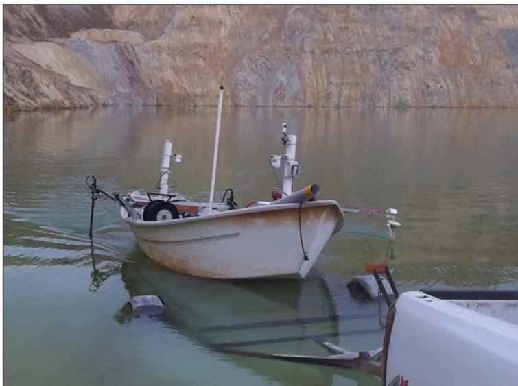
Figure 4. The aquatic drone craft that was developed by Montana Tech and the MBMG for remote sampling of Berkeley Pit water.
