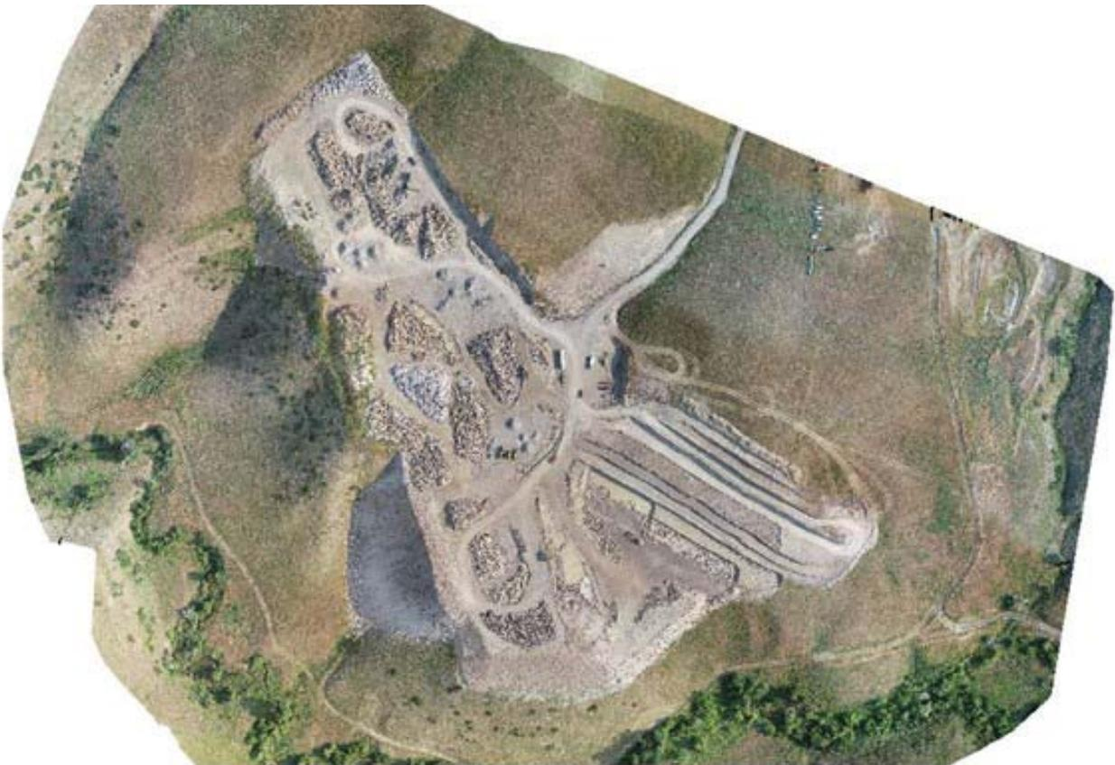
Figure 4. High-resolution orthomosaic map rendered by Pix4Dmapper using aerial imagery collected on site with UAV.
