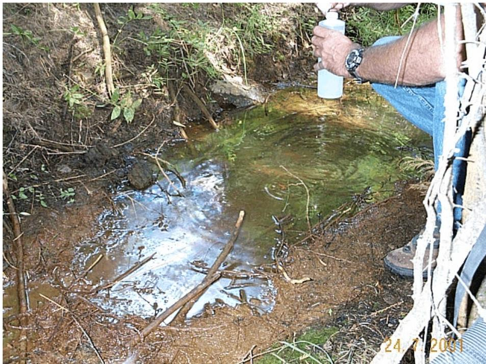
**Figure 24b.** Vulcan Tunnel's adit discharge had an oily sheen on the brightly orange-stained water.
