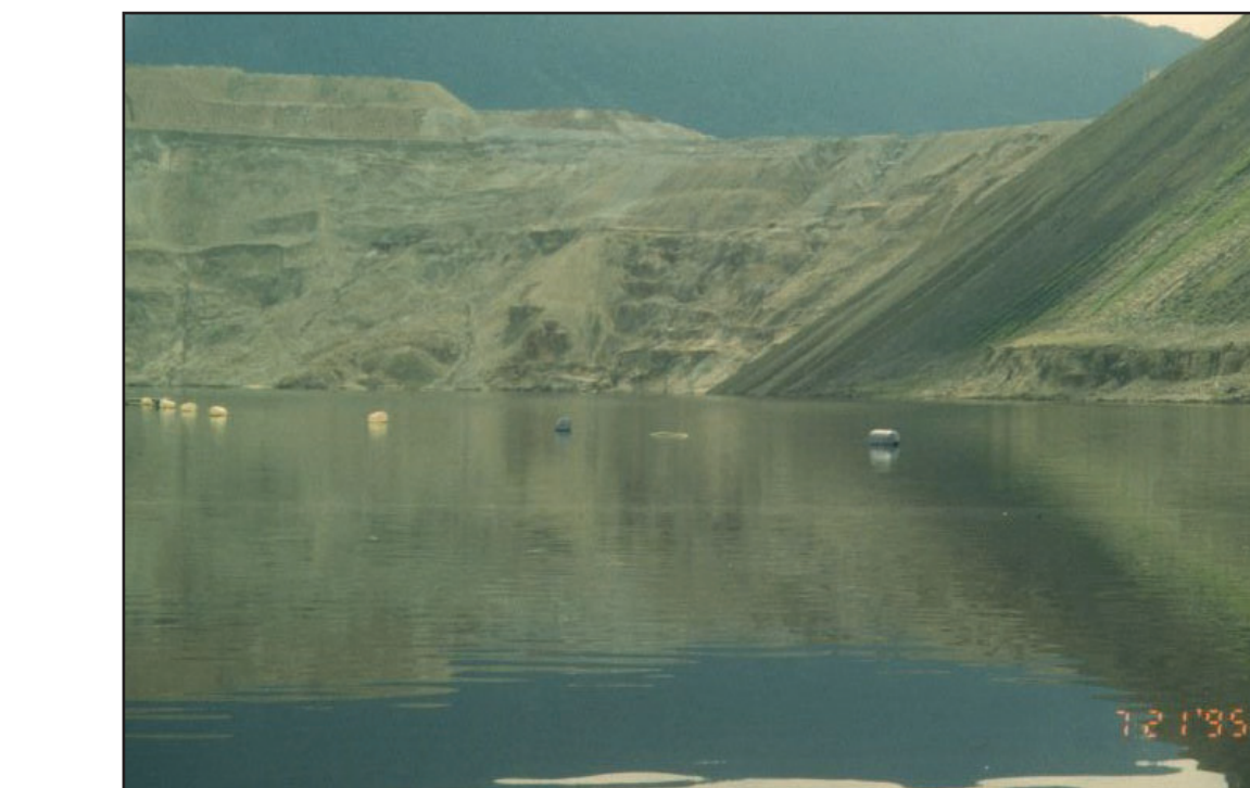
Figure 6. Floating barrels supporting sample tubing used for collection of bulk water samples.
