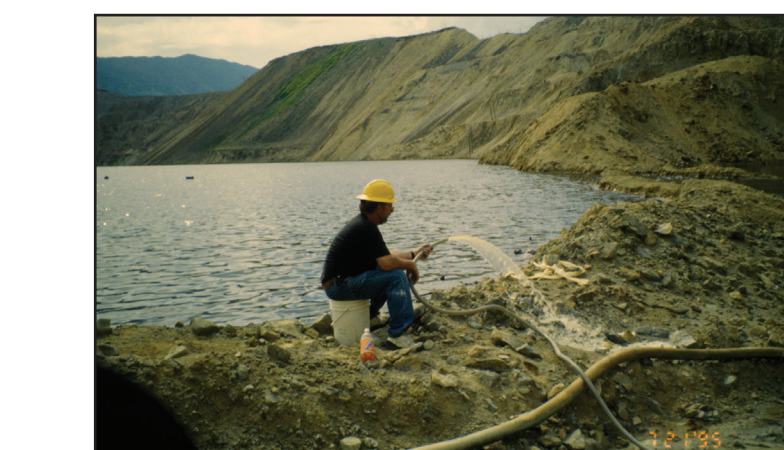
Figure 3. View looking northeast showing erosion of pit haul roads from surface-water discharge, September 1984.
