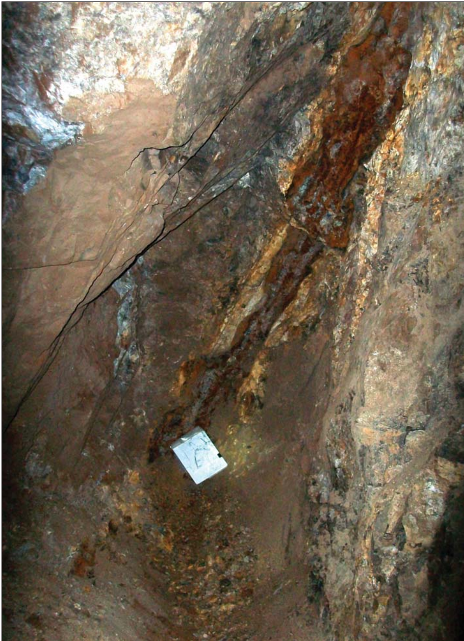
Figure 8. Photo of Hilltop vein at west face of main stope above 800 level; clipboard for scale.
