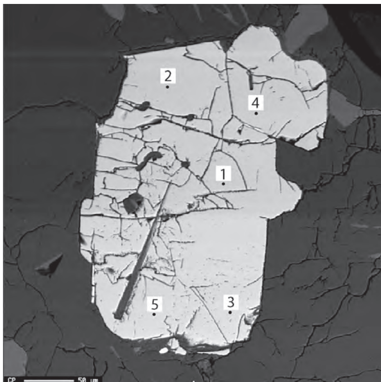
Figure 5. BSE image of gahnite grain with measured chemical composition. From an area of JA-04-32 with abundant sillimanite prisms, some retrograded to secondary muscovite. Matrix in image is predominantly quartz and feldspar. Small circles below numbers locate analyses. Scale bar is 50 \mu\text{m} .
